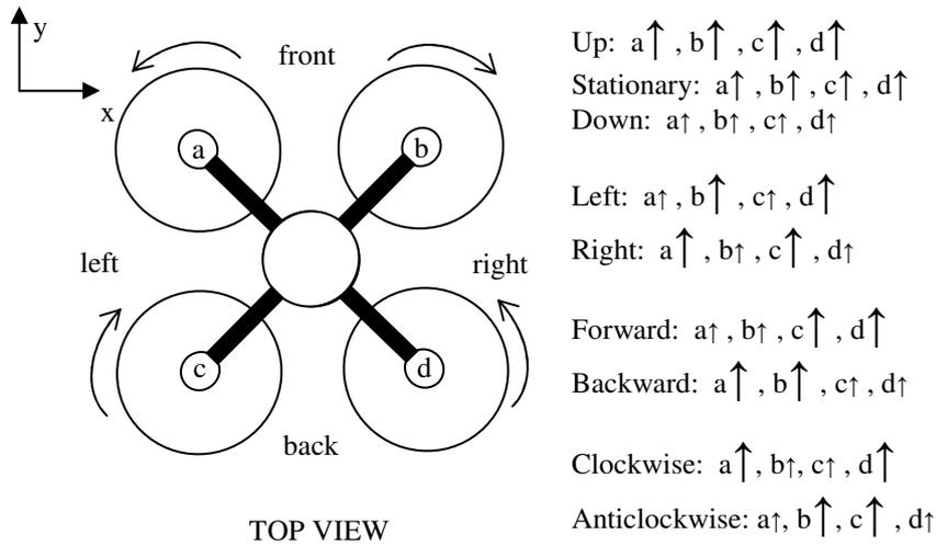
Fig. 4. “X” configuration for flight control (size of arrow is proportional to thrust)
