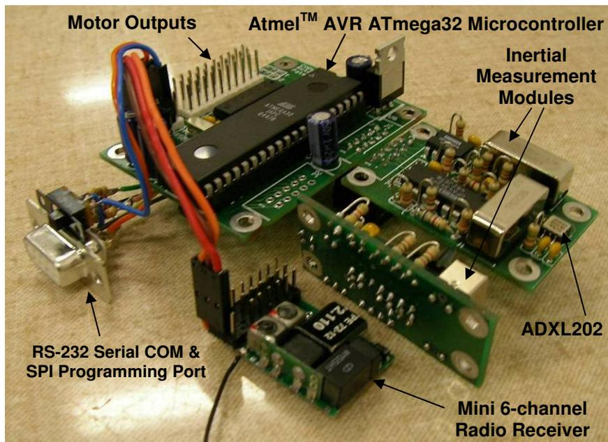
Fig. 8. Electronics Modules Laid Out Prior to Mounting
