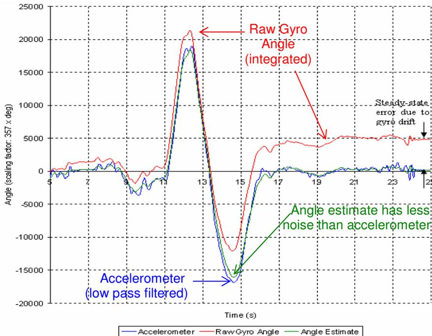
Fig. 10. Experimental Angle Estimation Data
