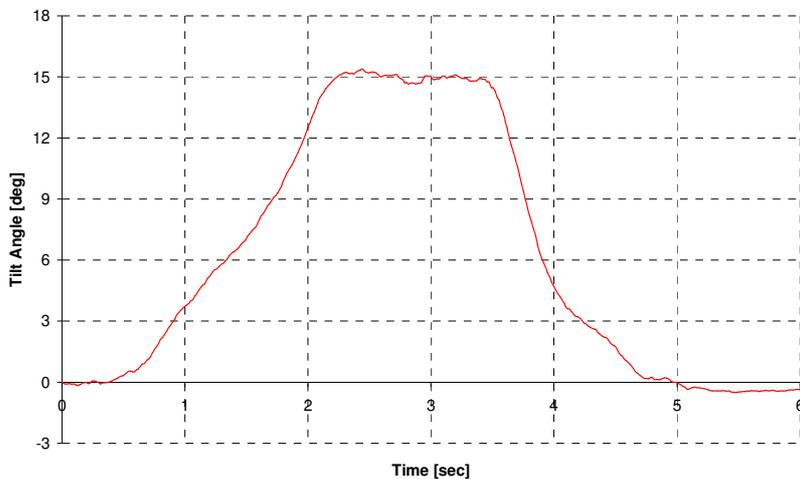
Fig. 11. Step Response with Tuned Controller Gains
