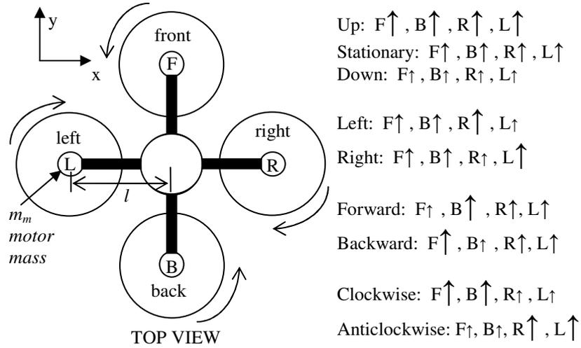
Fig. 3. Plus “+” configuration for flight control (size of arrow is proportional to thrust)
