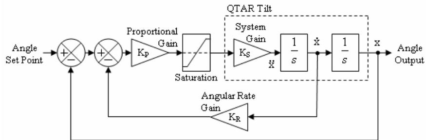
Fig. 5. Pitch/Roll Controller Block Diagram
