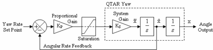
Fig. 6. Yaw Rate Controller Block Diagram
