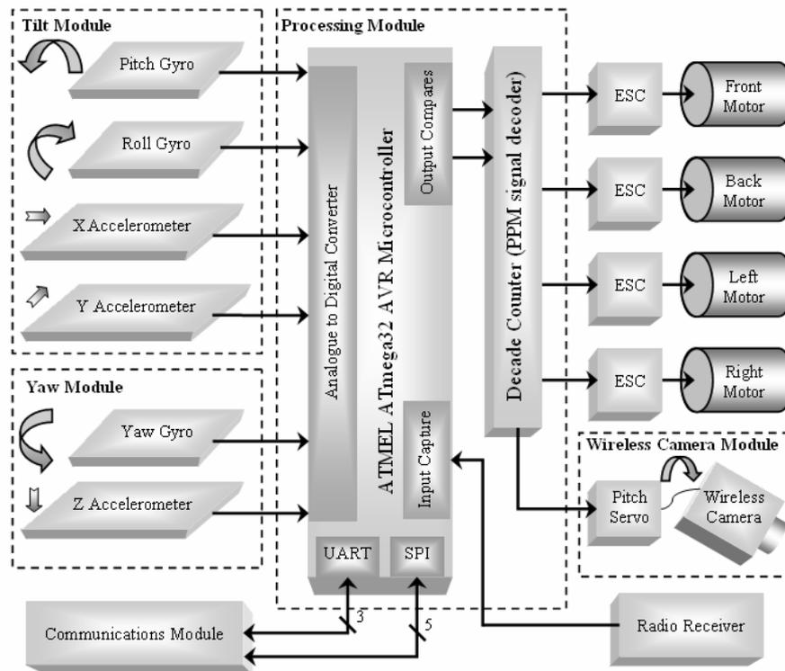
Fig. 7. QTAR Control Electronics Block Diagram
