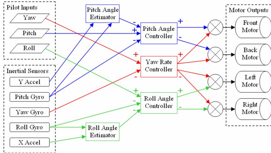
**Fig. 12.** Signal flow diagram for the QTAR ACS (Attitude Control System)
