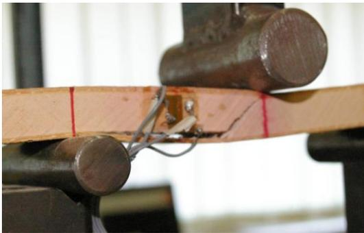
Figure 4. Failure behaviour of specimen AS-SW-F.
