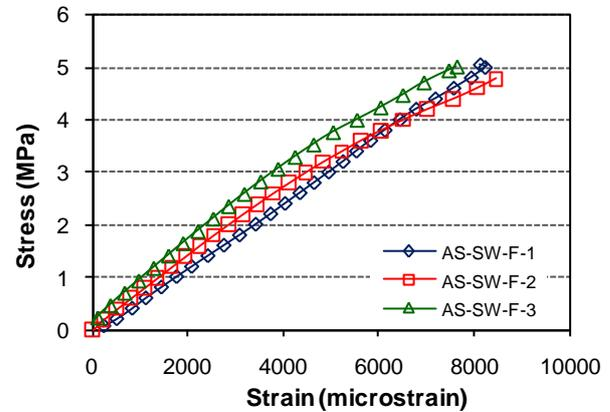
Figure 2. Shear stress-strain behaviour of specimen AS-SW-F.
