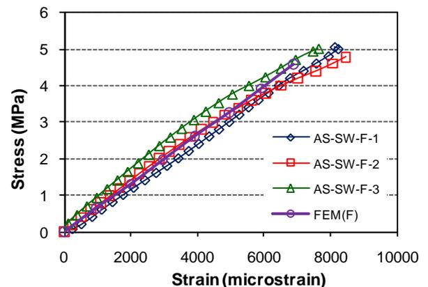
Figure 8. FEM and experimental shear stress-strain behaviour of specimen AS-SW-F.
