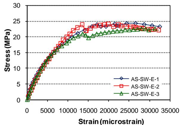
Figure 3. Shear stress-strain behaviour of specimen AS-SW-E.
