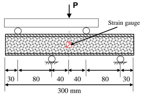
Figure 1. Illustration of asymmetrical beam shear test.
