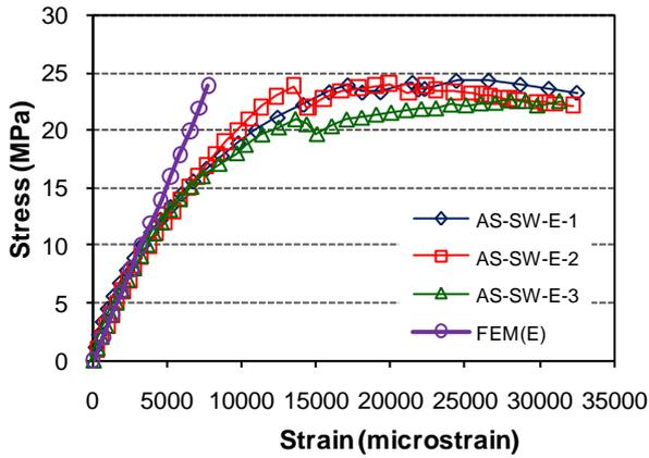
Figure 9. FEM and experimental shear stress-strain behaviour of specimen AS-SW-E.
