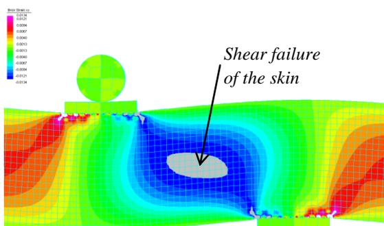
Figure 11. Predicted failure of AS-SW-E at a load of 17 kN.
