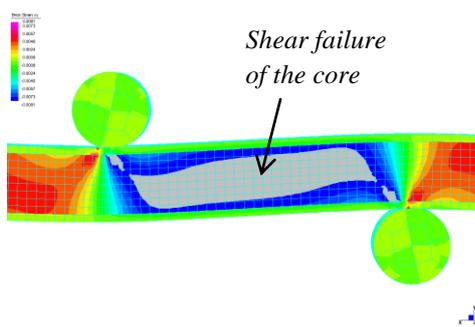
Figure 10. Predicted failure of AS-SW-F at a load of 10 kN.
