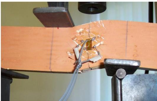
Figure 5. Failure behaviour of specimen AS-SW-E.
