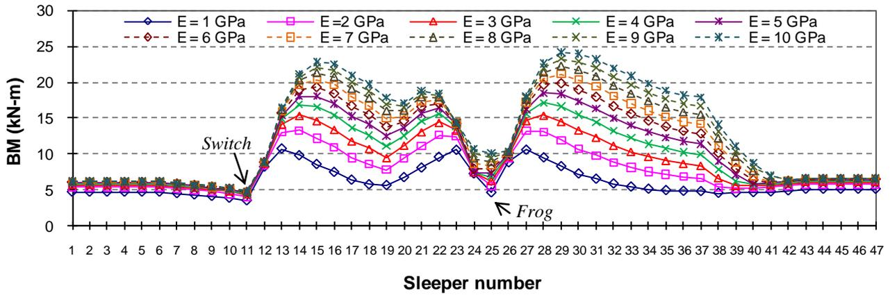
Figure 5. Positive bending moment when  $U_s = 10$  MPa.
