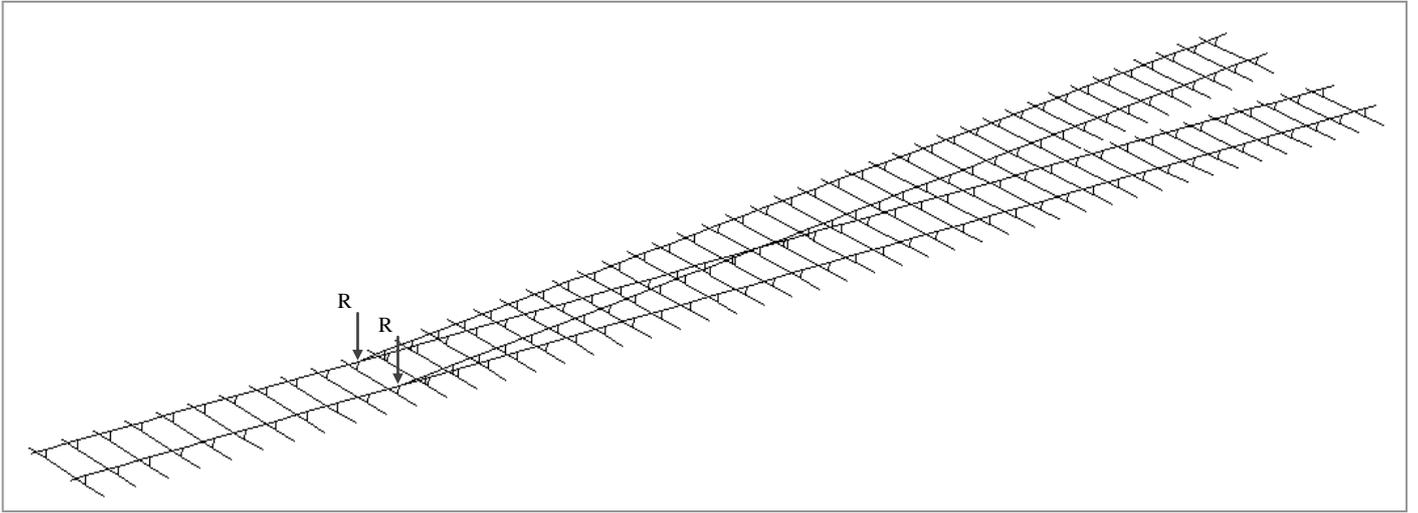
Figure 3. The grillage beam model for railway turnout.
