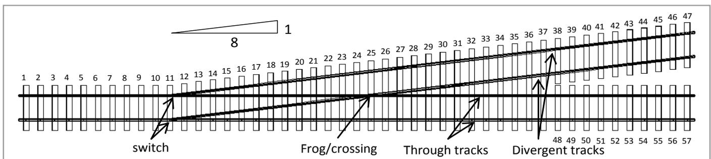
Figure 2. geometry of a 1:8 standard left-hand railway turnout.
