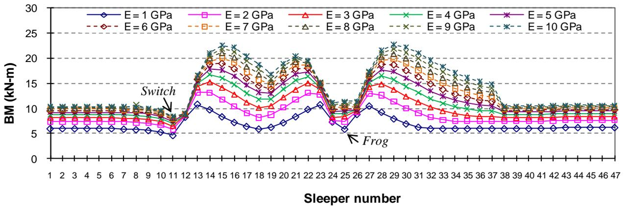
Figure 6. Positive bending moment when  $U_s = 40$  MPa.
