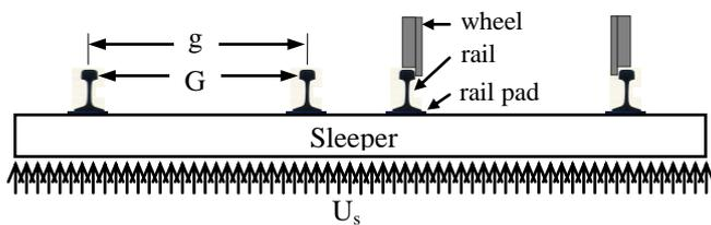
Figure 1. Schematic diagram of a turnout railway sleeper.
