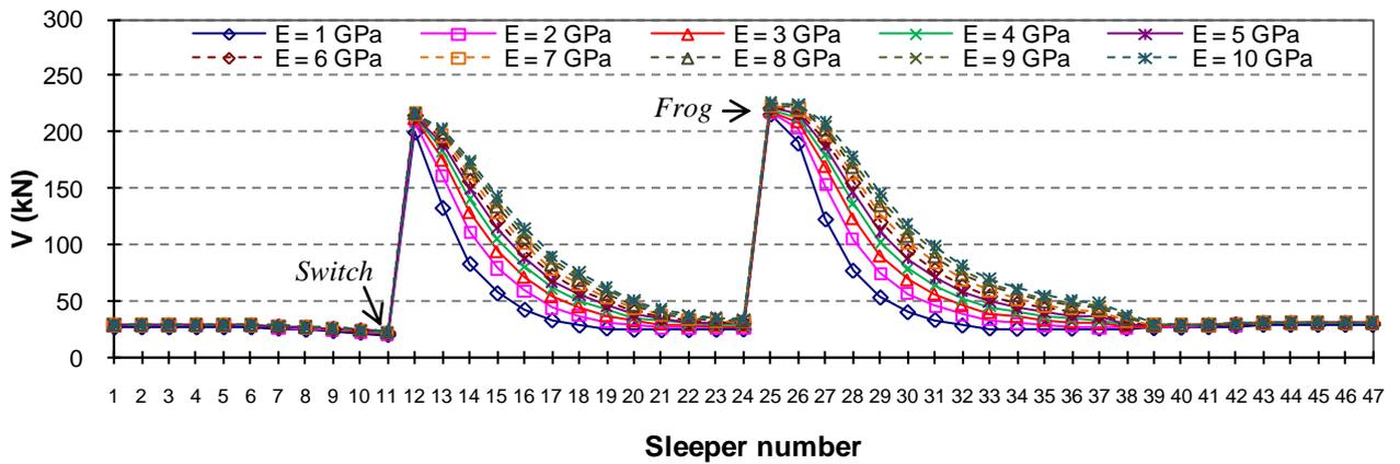
Figure 7. Maximum positive shear force when  $U_s = 10$  MPa.
