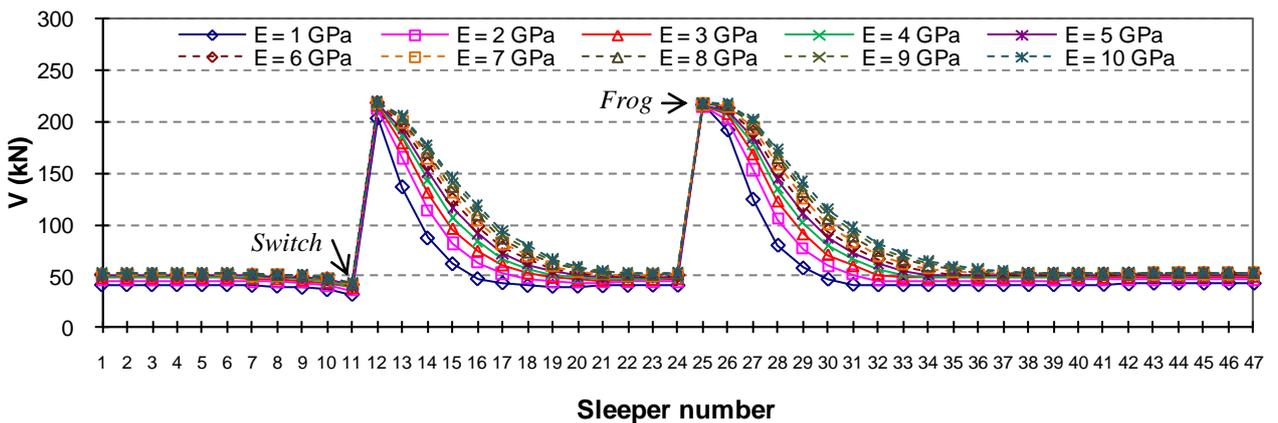
Figure 8. Maximum positive shear force when  $U_s = 40$  MPa.
