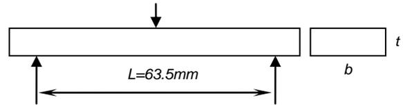
**Fig.1** Three-point loading for flexural tests.
