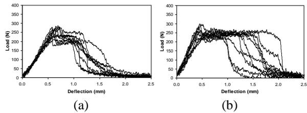
**Fig.9** Load-deflection curves from three-point flexural testing on sandwich composites for 30/1 water/starch ratio in interface between syntactic foam core and skin paper: (a) SL300WS30-W530; (b) SL75WS50-W530.
