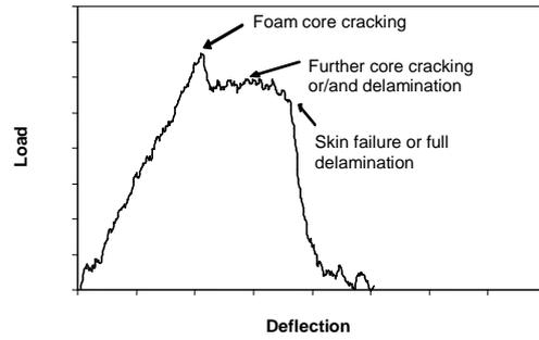
**Fig.8** Schematic for different stages of failure/damage process.
