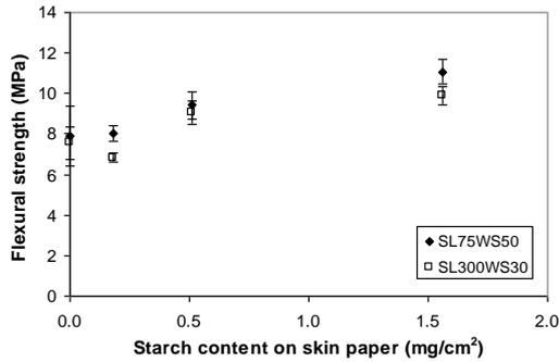
**Fig.6** Estimated flexural strength based on Eq. (2) for sandwich composites for different starch contents in adhesive contained in skin paper. The zero starch content is for syntactic foam core only without skin paper. The error bars indicate 95% confidence intervals.
