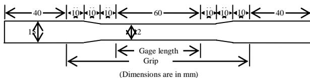
**Fig.2** Tensile test specimen for skin paper.
