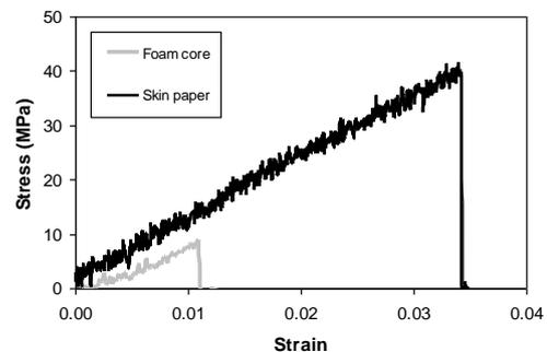
**Fig.3** Examples for flexural (maximum) stress versus maximum strain curve (in grey) obtained using Eq. (2) and (3) for syntactic foam panel SL75WS50; and for tensile stress strain curve (in black) obtained from skin paper without starch adhesive on.
