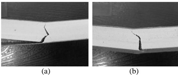
**Fig.7** Examples for delamination after fracture under three point flexural loading: (a) SL75WS50-W570, fully delaminated; and (b) SL75WS50-W514, least delaminated.
