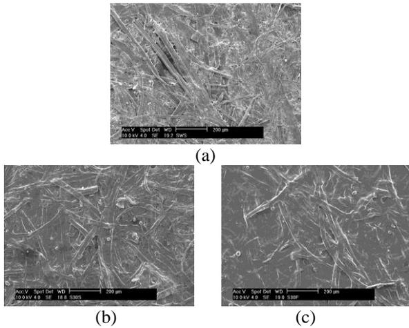
**Fig.5** SEM images of typical skin paper surfaces: (a) without starch adhesive; (b) coated with starch adhesive, slowly dried; and (c) coated with starch adhesive, fast dried.
