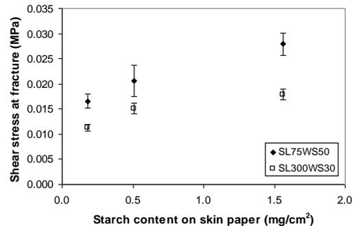
**Fig.10** Shear stress on interface between syntactic foam and skin paper calculated using Eq. (7) for different starch content on skin paper. The error bars indicate 95% confidence intervals.
