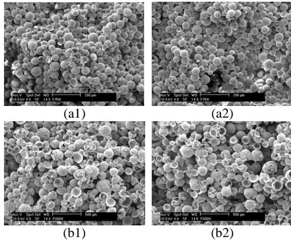
**Fig.4** Scanning electron microscopic (SEM) images of fracture surfaces of syntactic foam panels from three-point flexural tests: (a1) compression side of SL75-WS50; (a2) tension side of SL75WS50; (b1) compression side of SL300WS30; and (b2) tension side of SL300WS30.
