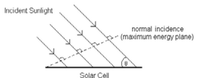
Figure 1: The energy captured by a solar cell depends on the intensity of the sunlight and the angle at which sunlight is incident upon the cell. The maximum energy is received when the sunlight is normally incident to the solar cell. The plane of maximum energy capture moves throughout the day as the sun traverses the sky.
