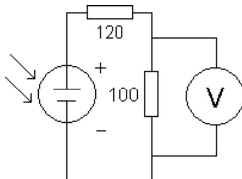
Figure 3: The maximum output of the external solar cell circuit is first measured by placing a voltmeter in parallel with the load resistor. Placing your hand over the cell should show that the cell is working correctly by noting an immediate drop in the output voltage.
