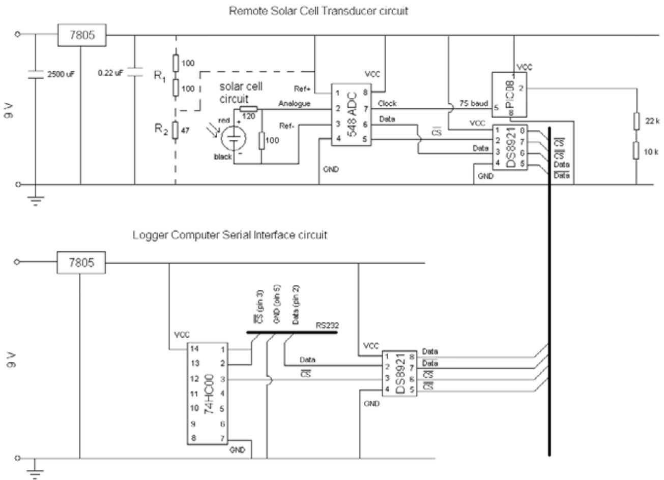
Figure 2: Circuit design and wiring diagram of the solar cell monitoring station.
