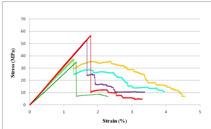
Figure 6. Stress-strain plot of flexural specimens of gomuti fibres/polyester composites: random-original
