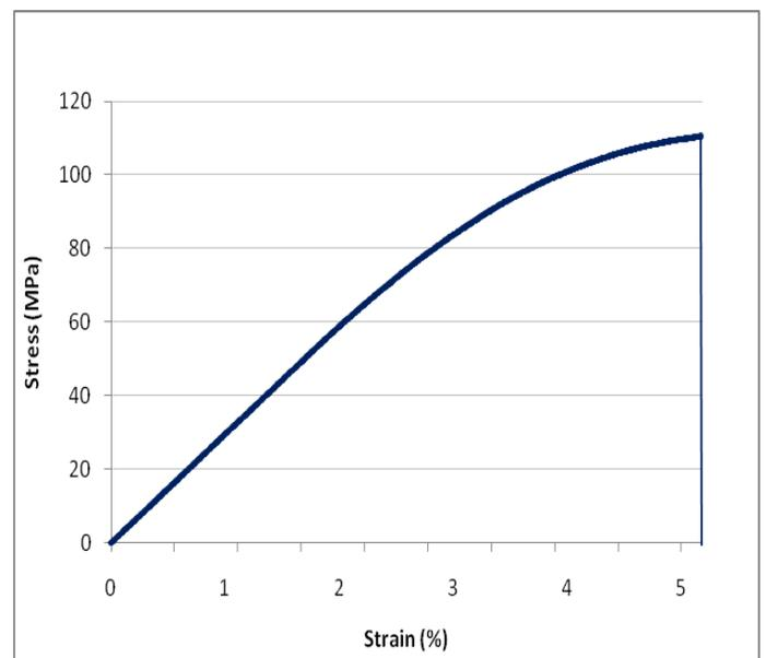
Figure 10. Stress-strain plot of neat polyester resin
