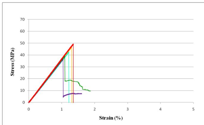
Figure 7. Stress-strain plot of flexural specimens of gomuti fibres/polyester composites: chopped
