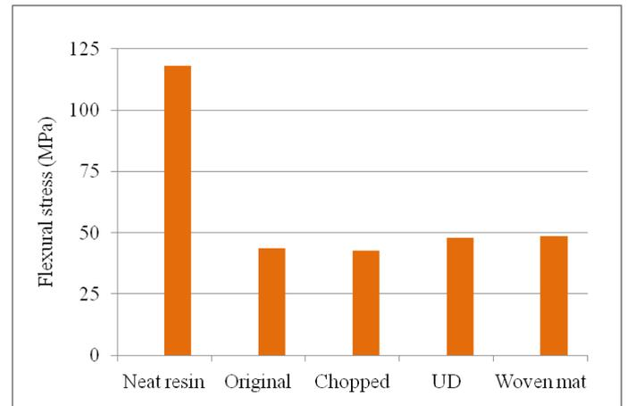
Figure 4. Tensile and flexural stress comparison
