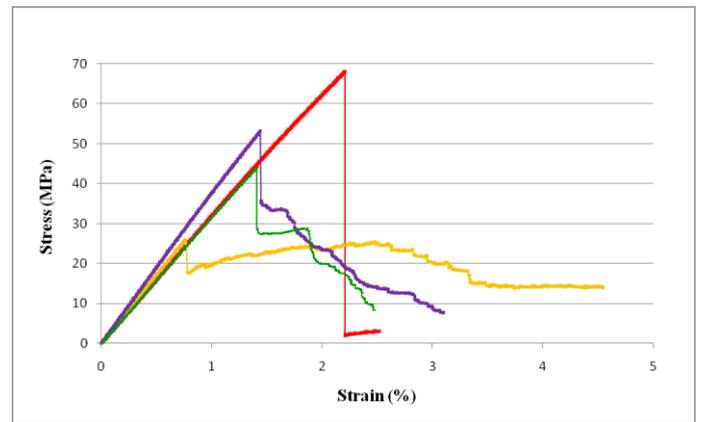
Figure 8. Stress-strain plot of flexural specimens of gomuti fibres/polyester composites: unidirectional
