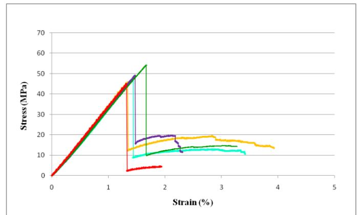
Figure 9. Stress-strain plot of flexural specimens of gomuti fibres/polyester composites: woven mat
