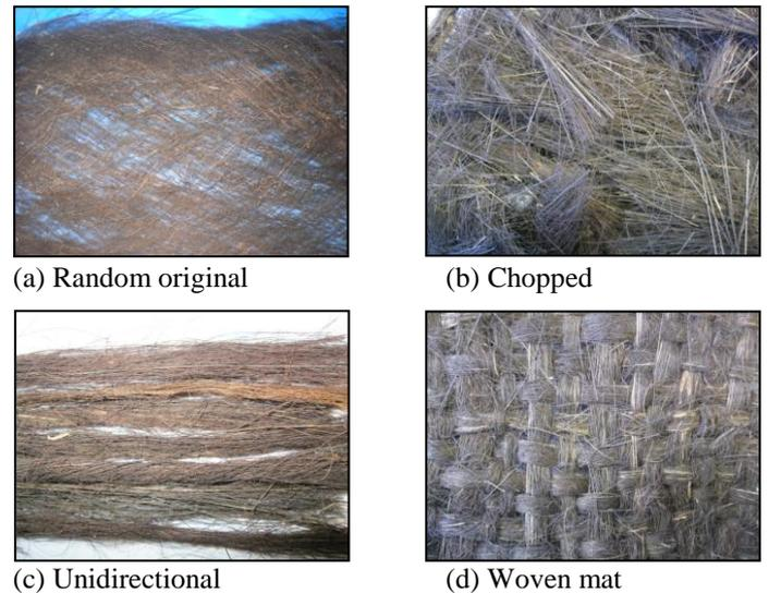
Figure 3. Orientation of the fibres
