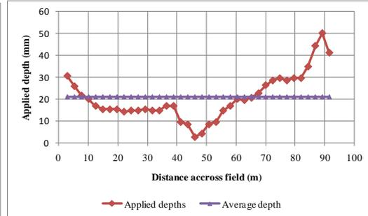
Fig. 3: Water distribution (overlap pattern, 90 m spacing) for a travelling gun
