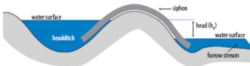
Fig. 2: Siphon operating with submerged flow (Source: Purcell 1994)
