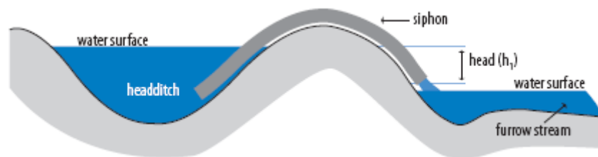
Fig. 1: Siphon operating with free flow (Source: Purcell 1994)
