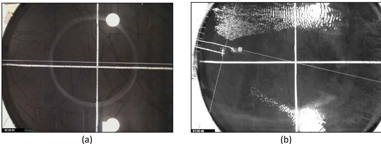
**Figure 4:** Images captured from video during large scale laboratory trials (performed on a 5.8m diameter test tank) to derive algorithms for monolayer spreading rate and dispersal angle: (a) Monolayer has been applied and is spreading under zero wind conditions in a linear circular shape, (b) Monolayer being applied continuously at 50 mL/min and dispersing in a wedge shape under an imposed uniform wind speed of 16.2 km/h.
