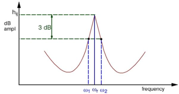
Figure 5 Half power method for damping estimation
