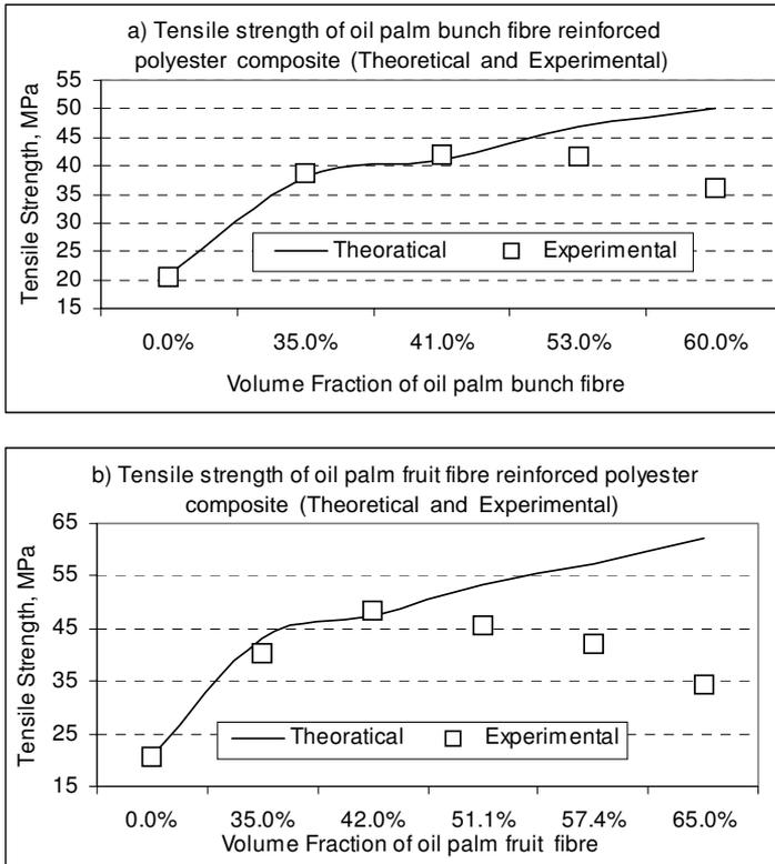
Fig. 7. Theoretical and experimental results of tensile strength against fibre volume fraction.
