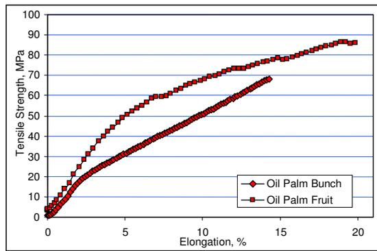
Fig. 2. Stress/strain diagram of single fibre.
