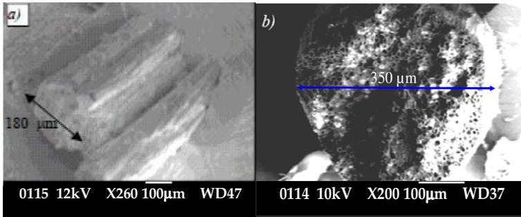
Fig. 1. SEM micrograph showing the two types of oil palm fibres as (a) fruit fibre and (b) bunch fibre.
