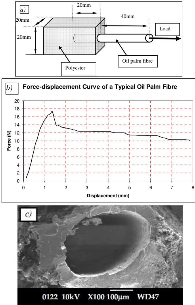
Fig. 3. Single fibre pull-out showing (a) schematic drawing describing pull out test and (b) pull-out force displacement curve of oil palm fibre (c) micrographs of the sample after test.
