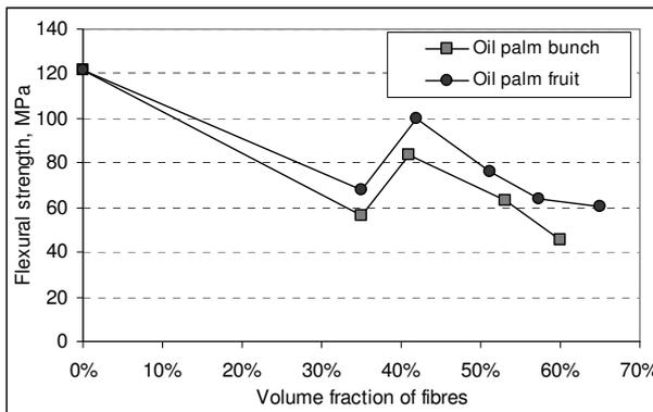
Fig. 9. Flexural strengths at the break of the composites at different fibre volume fractions.
