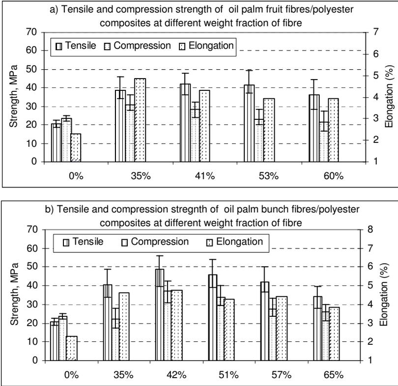
Fig. 4. Tensile and compression strengths associated with elongation (at the break) of the composites in different fibre volume fractions.
