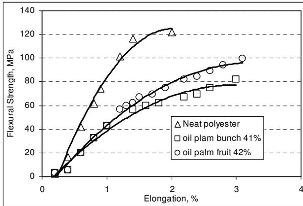
Fig. 8. Flexural stress-strain curves of the composites and neat polyester.
