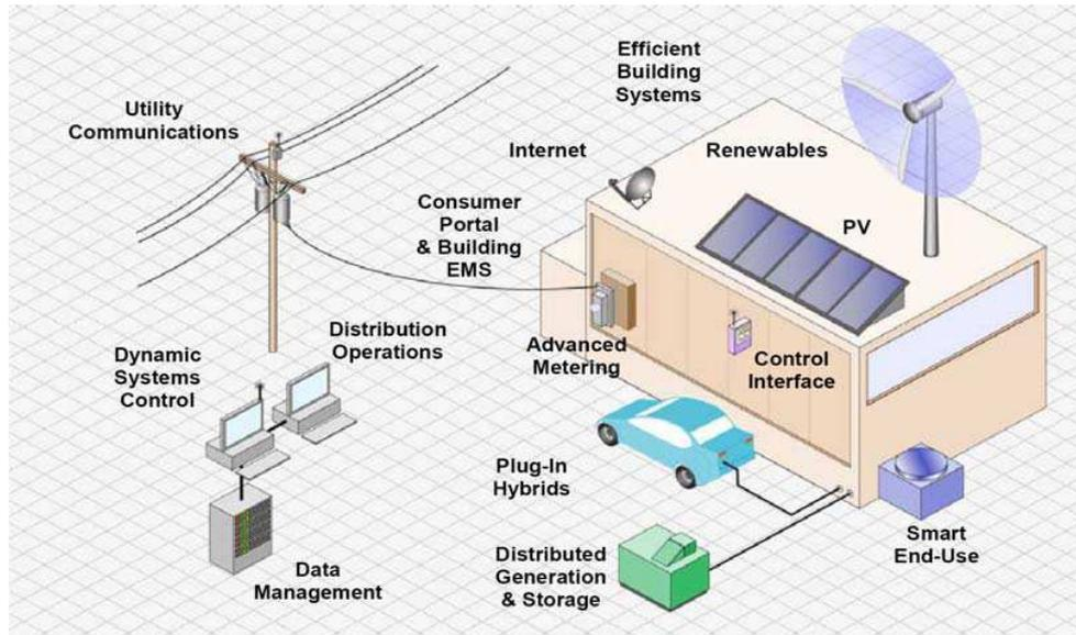
**Fig. 3:** Smart grid network diagram as said by Gellings, Clark W (2008)
