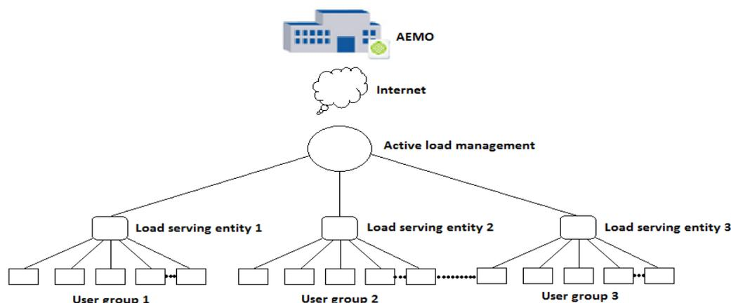
**Fig. 5:** Two-tier smart grid network architecture
