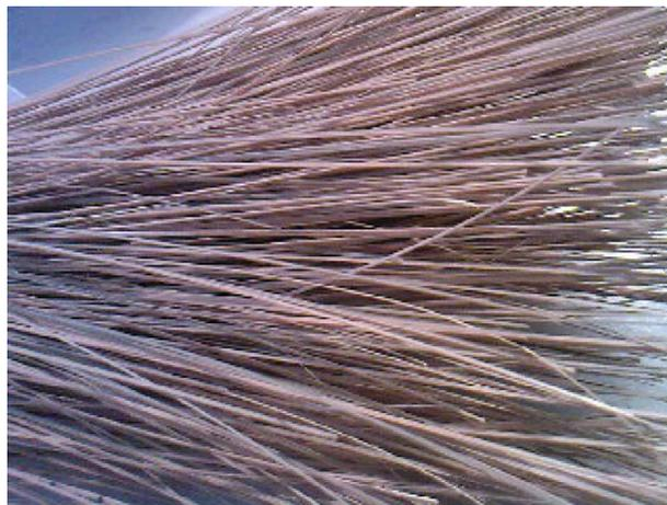
Fig. 1 Bamboo fibres used in this study
