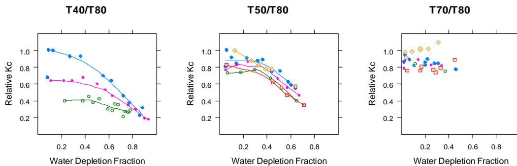
Figure 1. Relative wheat crop coefficient (Kc) of three deficit-irrigated treatments (T40, T50 and T70) with respect to a fully-irrigated treatment (T80) as a function of soil water depletion fraction measured in a greenhouse. (FC=0 WDF, pwp=1 WDF). Points and lines of different colors represent different soil drying cycles.
