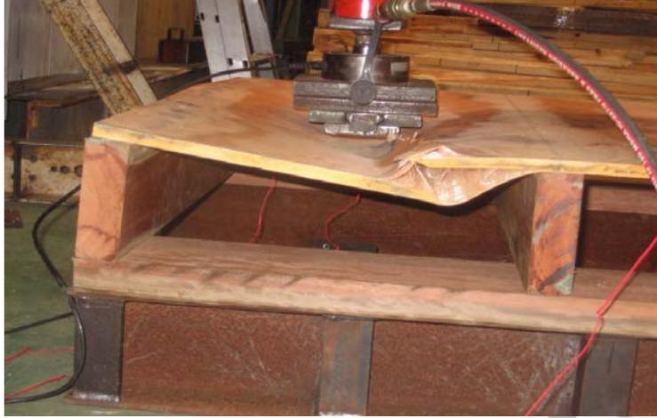
Fig. 4. Ultimate failure of two edges supported slab from delamination between skin and core
