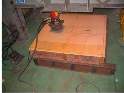
(b) Four edges supported slab testing
