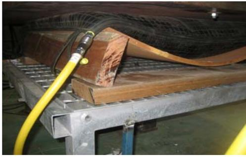
(a) Joist buckling
