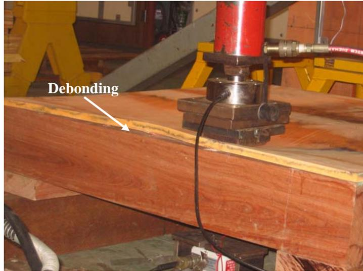
Fig. 11. Debonding failure between sandwich core and skins
