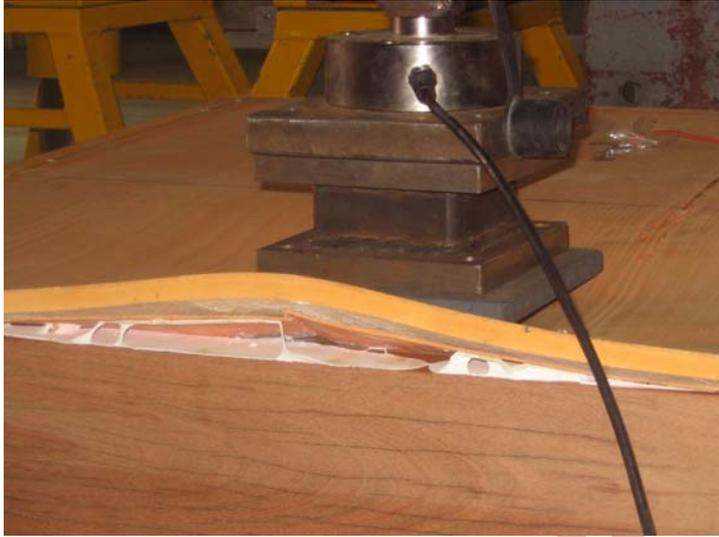
Fig. 5. Glue separation from joist and panel under point load
