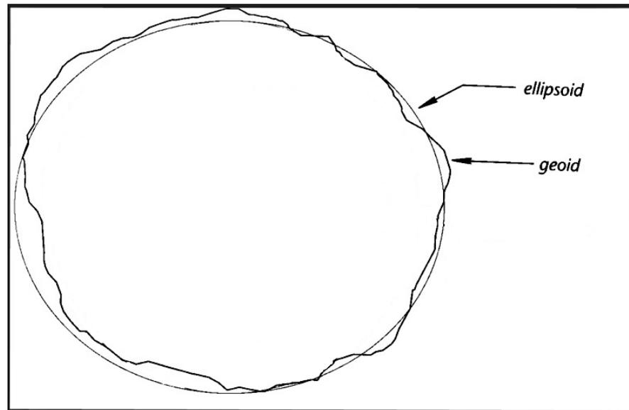
Figure 2.2 Relationship between ellipsoids and geoids
