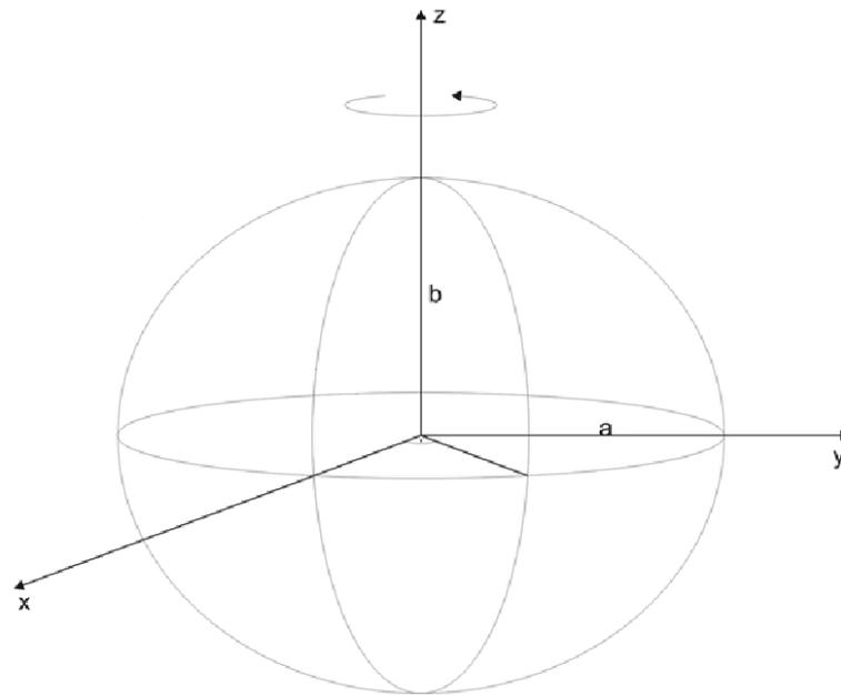
**Figure 2.1 A** Geocentric ellipsoid
