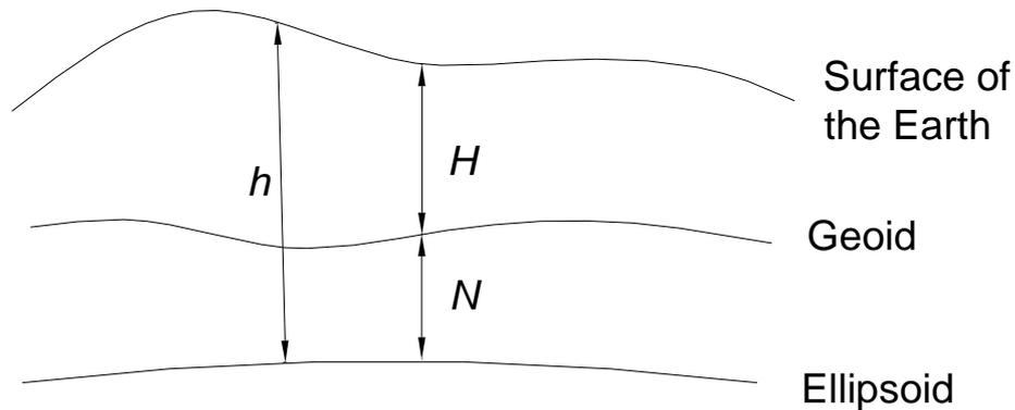
**Figure 2.3.** Relationship between Ellipsoid, Geoid and Orthometric Heights.
