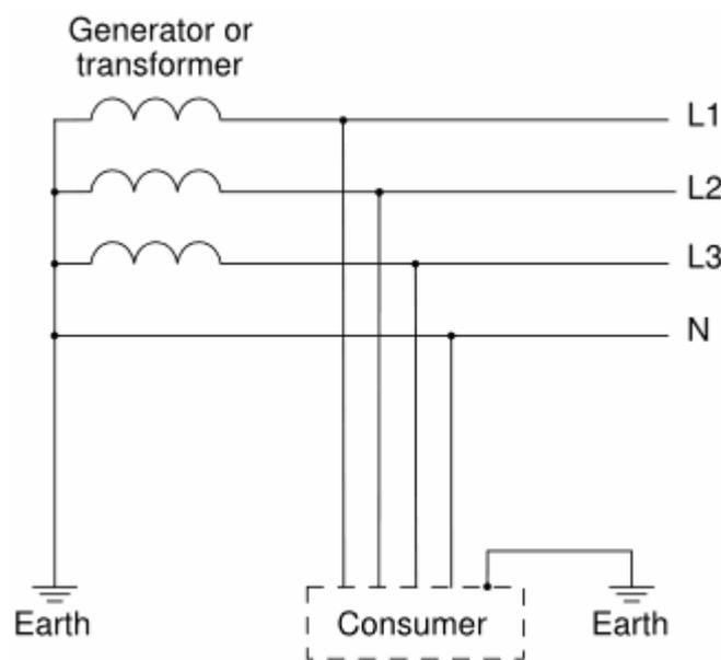
**Figure 2:** TT Earthing System. Note direct connection of supply source to Earth, as well as consumer equipment, but no connection between N-E at consumer terminals
