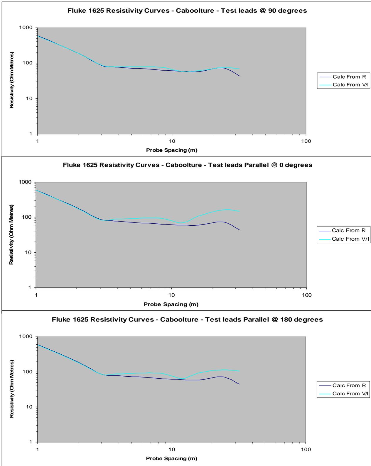
**Figure 19:** Resistivity Curves. Fluke 1625 - Caboolture Site: Resistivity curves as calculated from Resistance readings Vs measured Current and Voltage.
