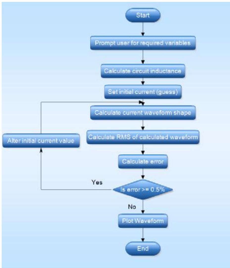
**Figure 33:** Program flowchart for calculation of R-L circuit current waveform
