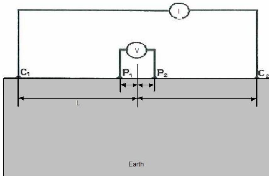
**Figure 7:** Schlumberger Array. Probe layout and injected and measured signals
