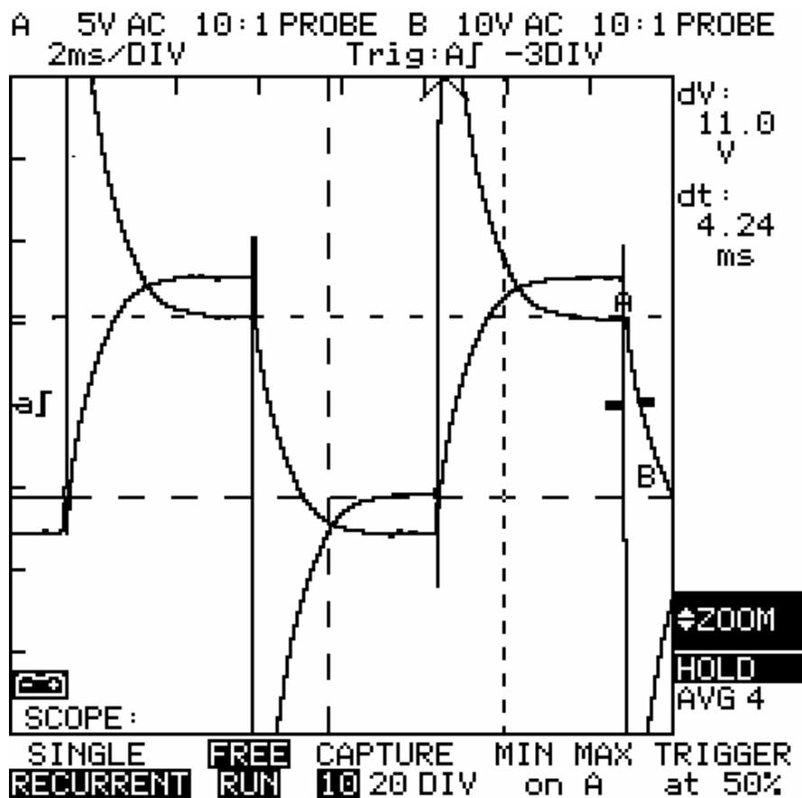
**Figure 28:** Voltage and Current Waveforms for Resistivity test with probe spacing of 150m, test leads in parallel Ch A: Measured Voltage, Ch B: Injected Current
