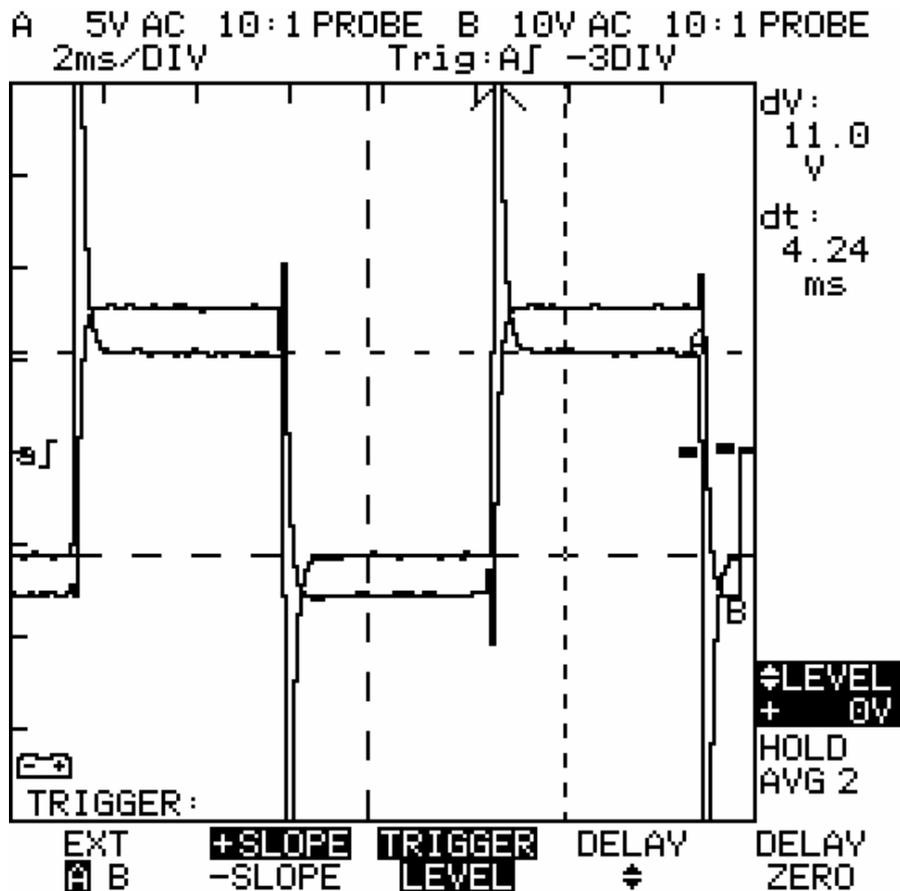
**Figure 29:** Voltage and Current Waveforms for Resistivity test with probe spacing of 150m, test leads 90° separated. Ch A: Measured Voltage, Ch B: Injected Current
