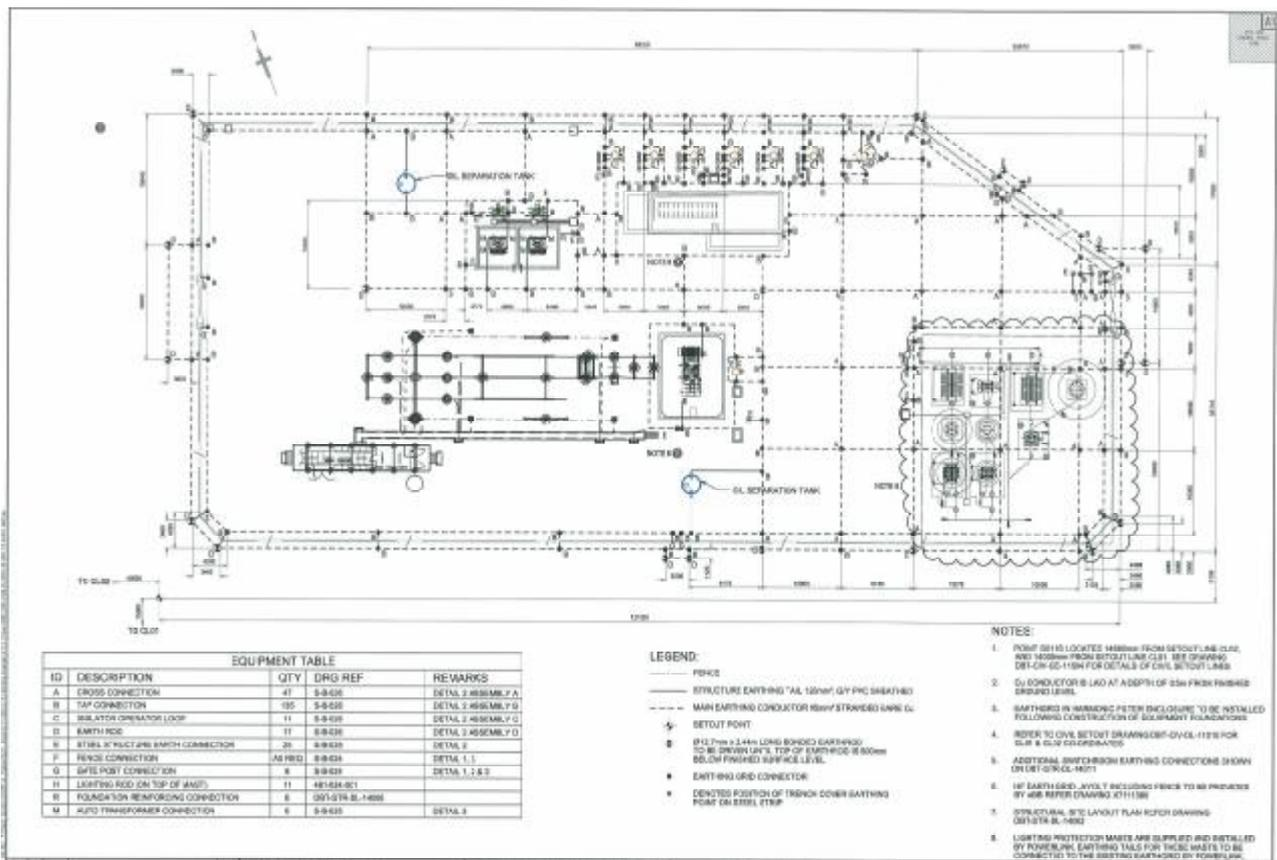
**Figure 1:** Example of a High Voltage Substation Earthing Grid (Reproduced with permission of Downer EDI Engineering)
