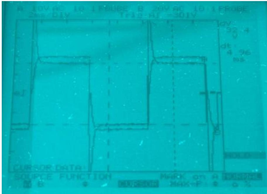
**Figure 22:** Voltage and Current Waveforms, 90° Test lead Orientation:
