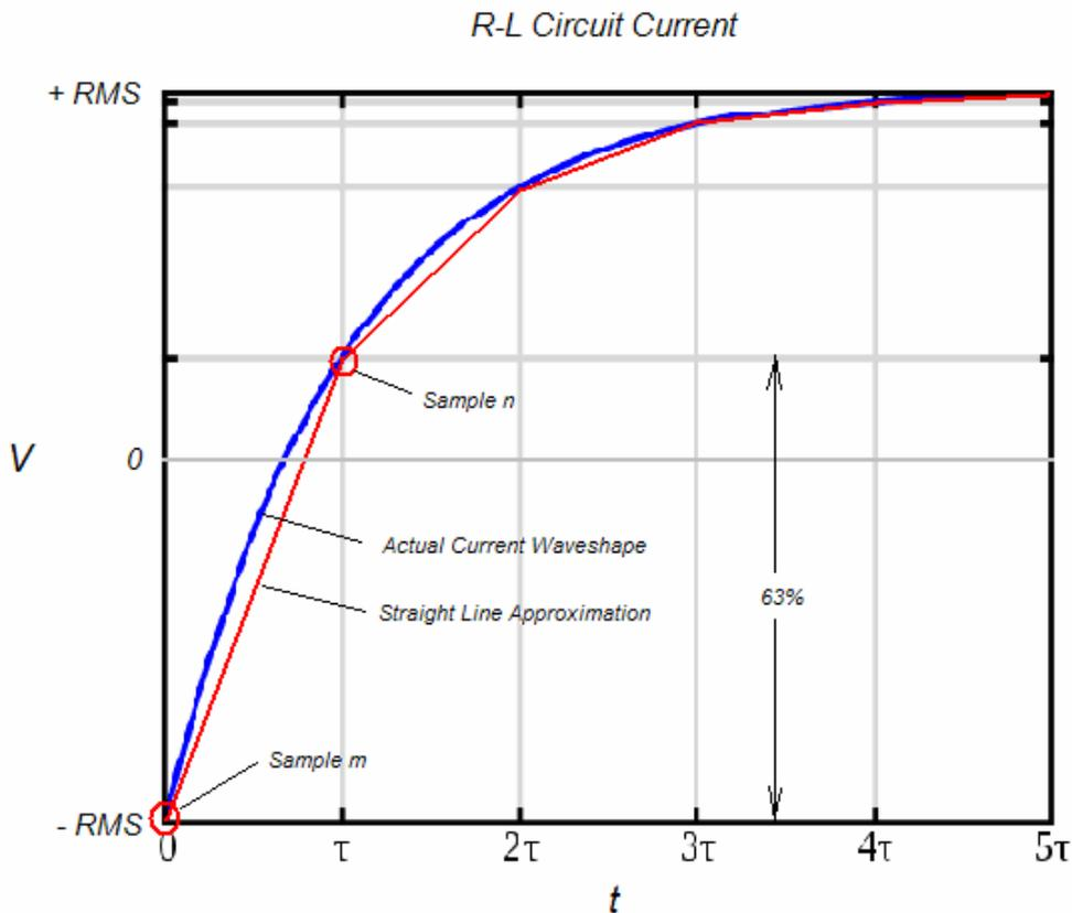
**Figure 32:** R-L Circuit current showing actual and calculated curve characteristics
