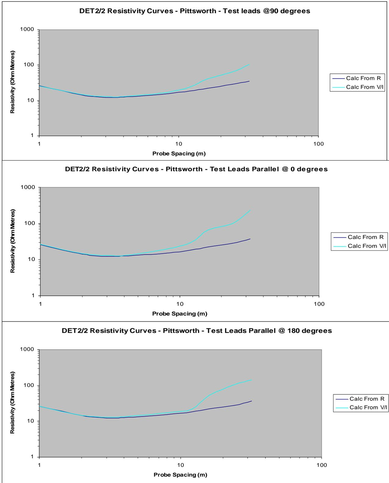
**Figure 20:** Resistivity Curves. Megger DET2/2 - Pittsworth Site: Resistivity curves as calculated from Resistance readings Vs measured Current and Voltage.
