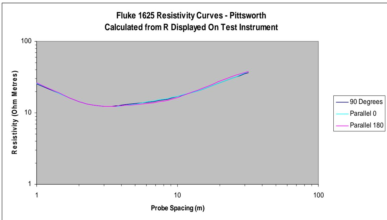
**Figure 17:** Resistivity Curves. Fluke 1625 - Pittsworth Site: Resistivity curves as calculated from resistance readings- Fluke 1625 instrument at Pittsworth site.
