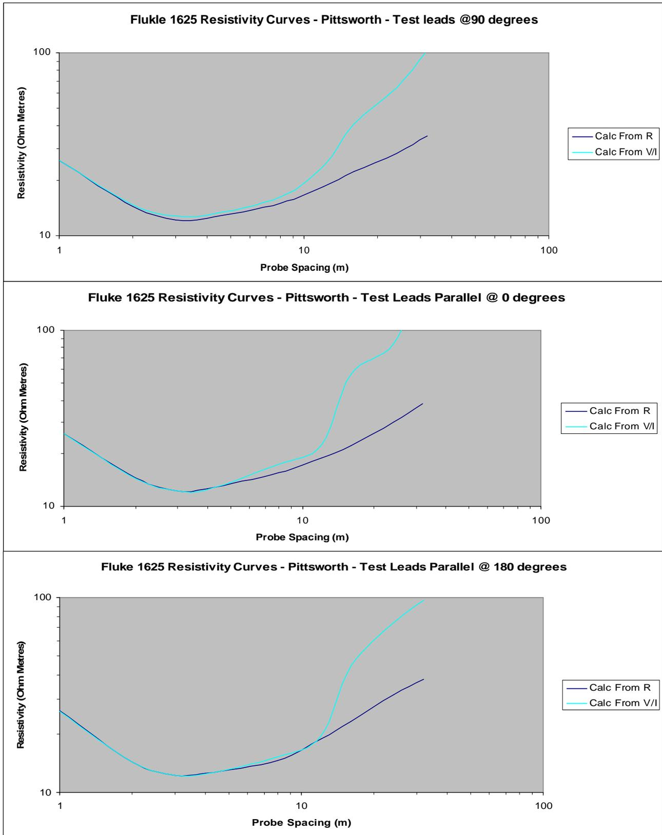
**Figure 21:** Resistivity Curves. Fluke 1625 - Pittsworth Site: Resistivity curves as calculated from Resistance readings Vs measured Current and Voltage.
