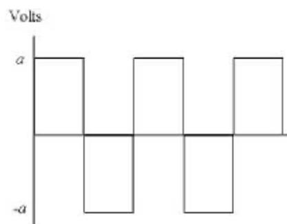
**Figure 13:** Example Square Wave: Example of a typical square wave, as is the injected current and measured voltage signal of the Fluke 1625 and Megger DET2/2.
