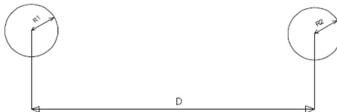
**Figure 31:** 2 Wire transmission line
