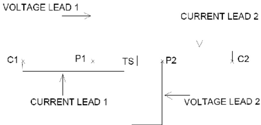
**Figure 9:** Test Leads at 90°. Wenner array with current and voltage leads separated by 90 degrees.
