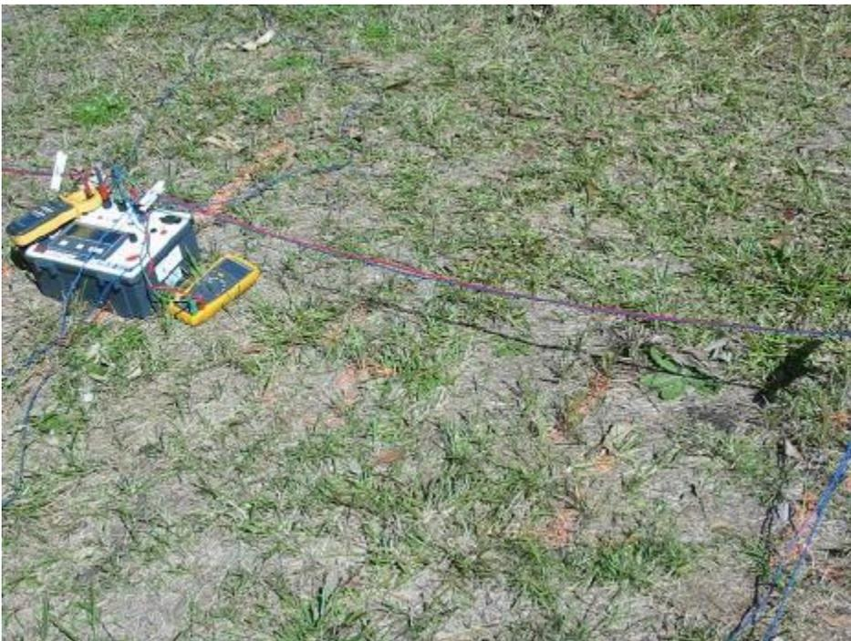
**Figure 12:** Parallel Test Lead Configuration : Wenner array with current and voltage leads in parallel.
