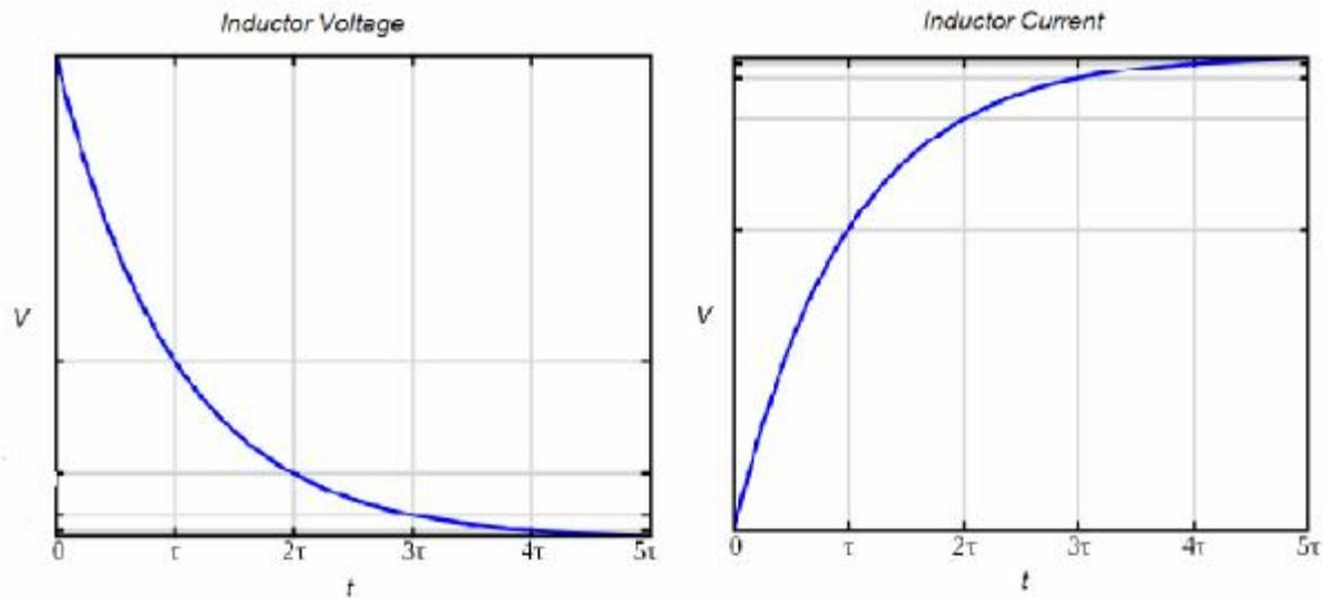
**Figure 27:** Typical Inductive Voltage and Current Waveforms for a voltage applied at time  $t=0$
