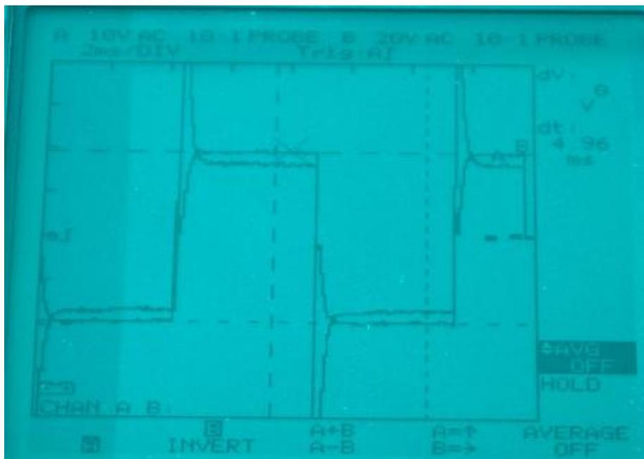
**Figure 23:** Voltage and Current Waveforms, Parallel 0° Test lead Orientation:
