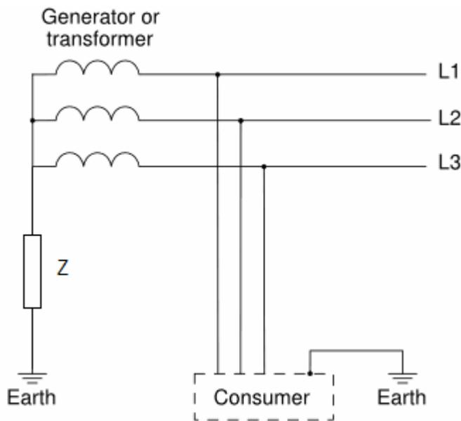
**Figure 4:** IT Earthing System. Note connection of supply source to Earth via an impedance, Z.
