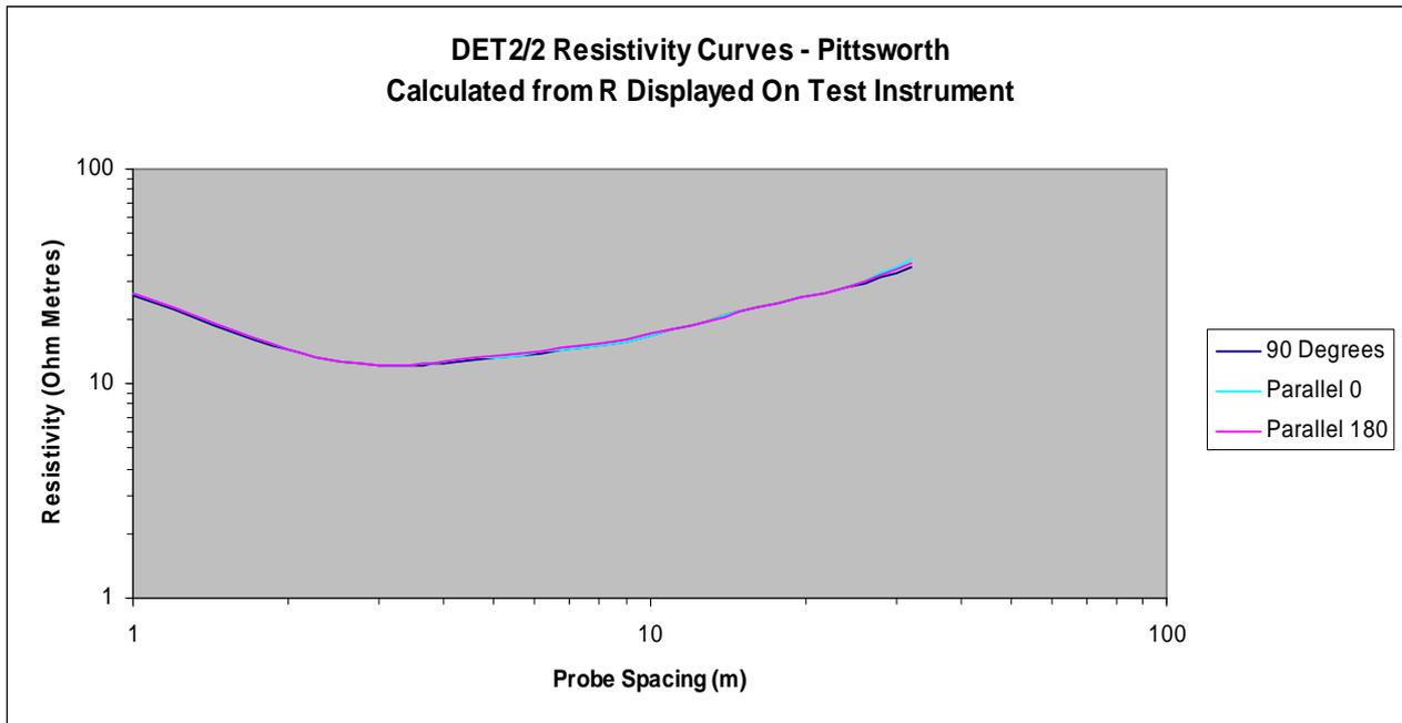
**Figure 16:** Resistivity Curves. DET2/2 - Pittsworth Site: Resistivity curves as calculated from resistance readings- Megger DET2/2 instrument at Pittsworth site.
