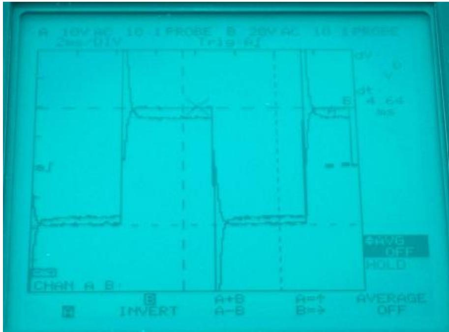
**Figure 24:** Voltage and Current Waveforms, Parallel 180° Test lead Orientation
