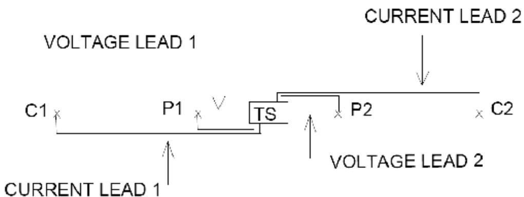
**Figure 10:** Test Leads in Parallel (0°). Wenner array with current and voltage leads in parallel (0 degrees).
