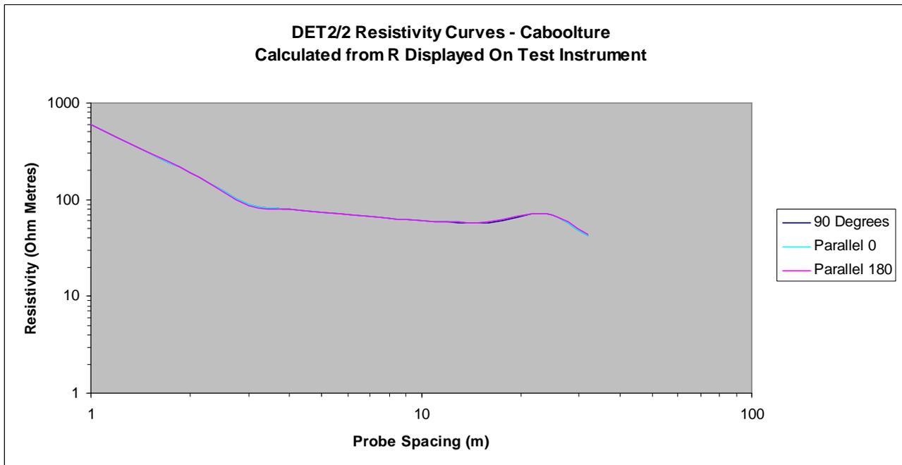
**Figure 14:** Resistivity Curves. DET2/2 - Caboolture Site: Resistivity curves as calculated from resistance readings- Megger DET2/2 instrument at Caboolture site.
