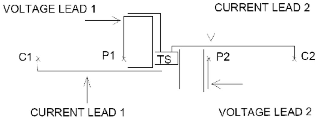
**Figure 11:** Test Leads in Parallel (180°). Wenner array with current and voltage leads in parallel (180 degrees).
