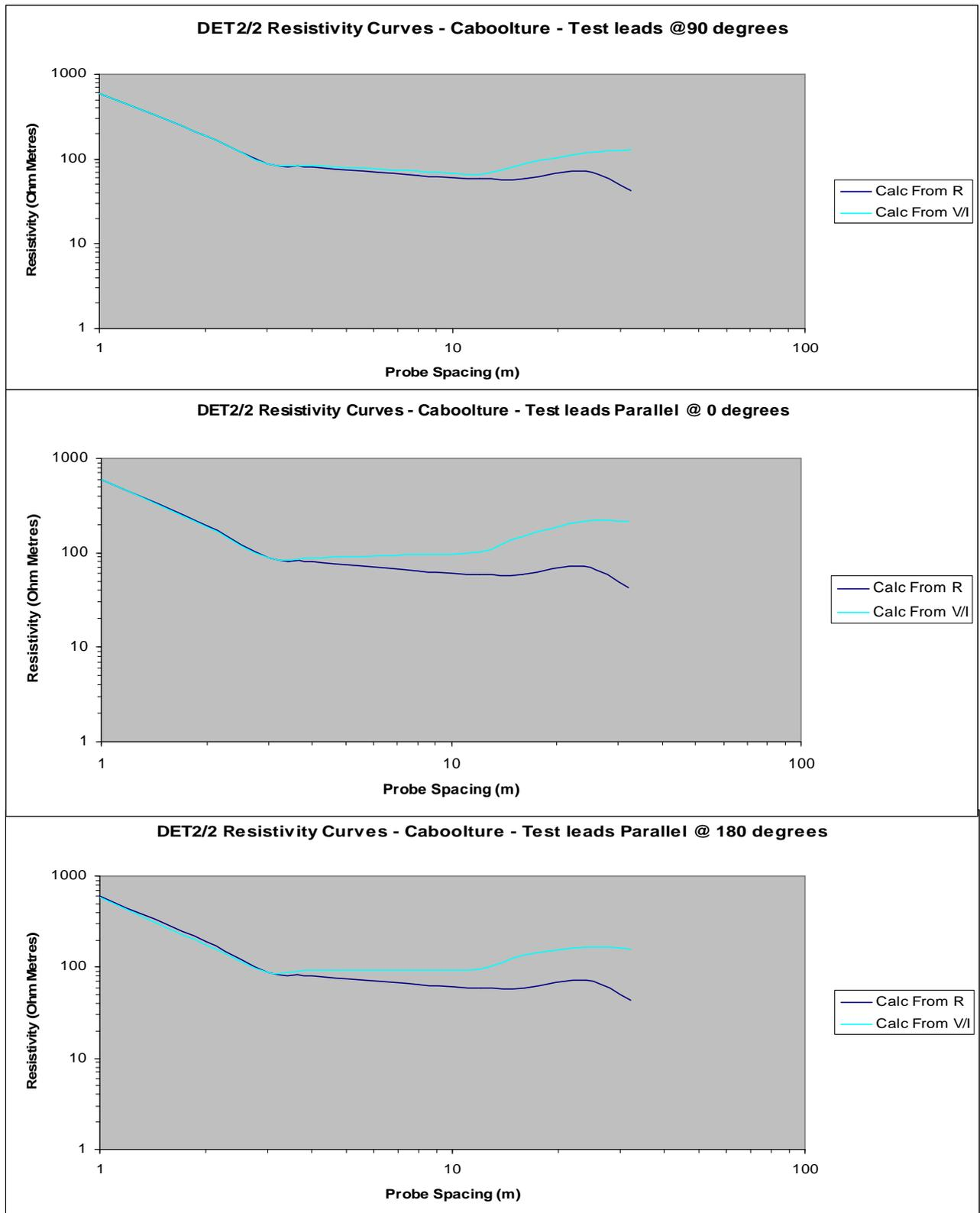
**Figure 18:** Resistivity Curves. Megger DET2/2 - Caboolture Site: Resistivity curves as calculated from Resistance readings Vs measured Current and Voltage.
