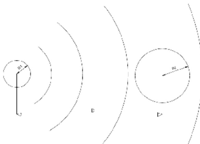
**Figure 30:** 2 Wire transmission line and magnetic field due to current in one conductor only
