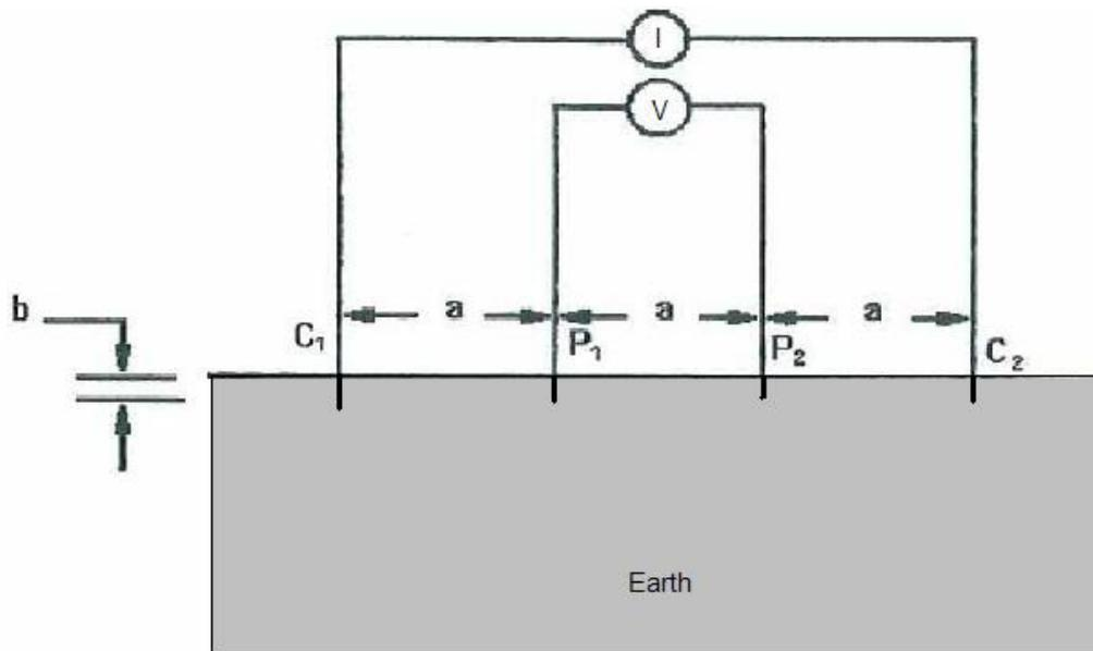
**Figure 6:** Wenner Array. Probe layout and injected and measured signals.
