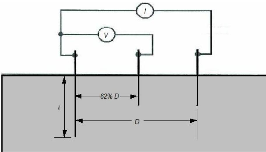
**Figure 8:** 3 Pin Array. Probe layout and injected and measured signals
