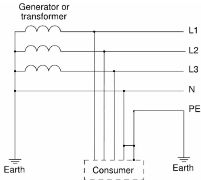
**Figure 3:** TN Earthing System. Note direct connection of supply source to Earth, as well as neutral conductor connection to earth at source and consumer terminals.
