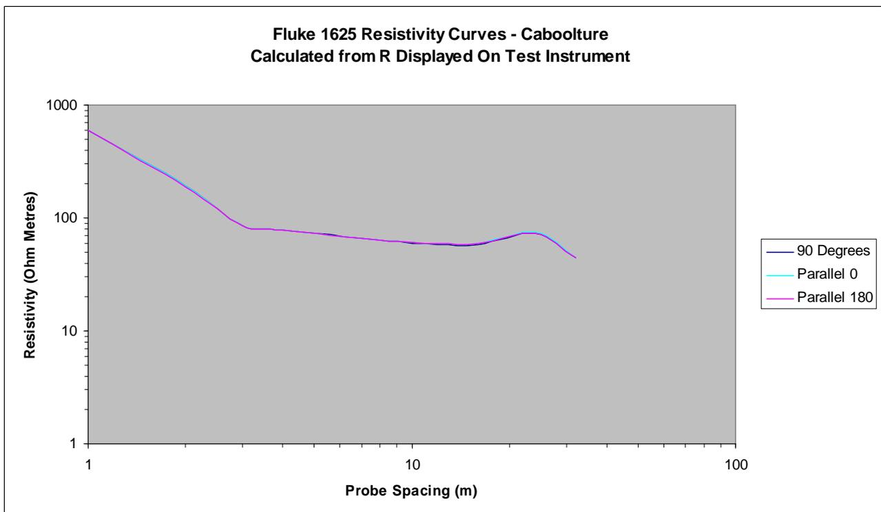
**Figure 15:** Resistivity Curves. Fluke 1625 - Caboolture Site: Resistivity curves as calculated from resistance readings- Fluke 1625 instrument at Caboolture site.
