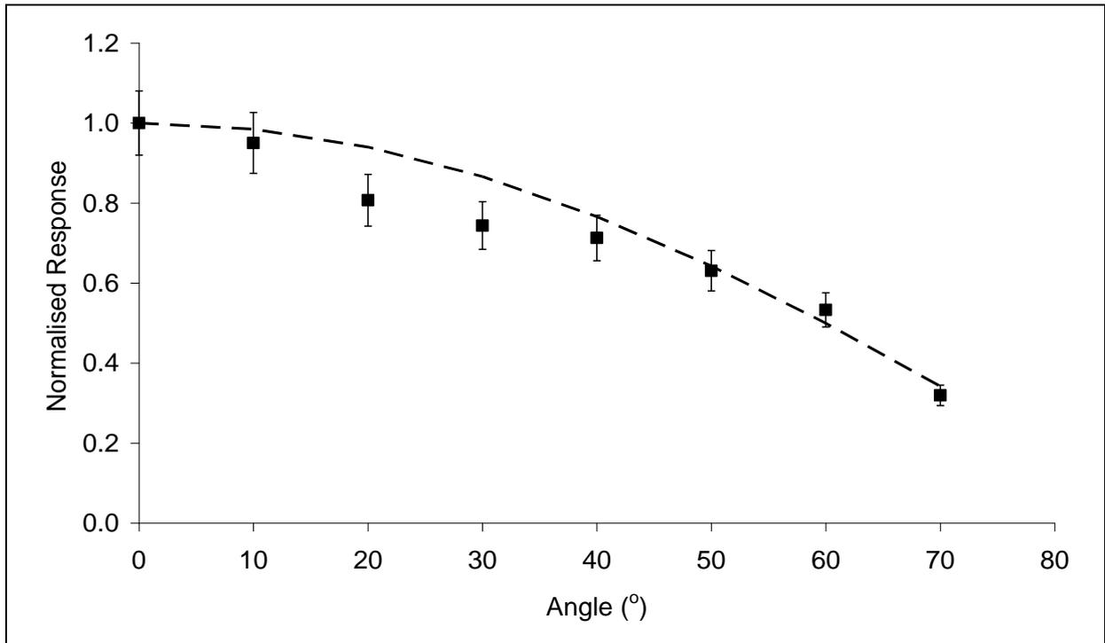
Figure 3. Comparison of the cosine response of the UV<sub>Mel</sub> dosimeter to the cosine curve.
