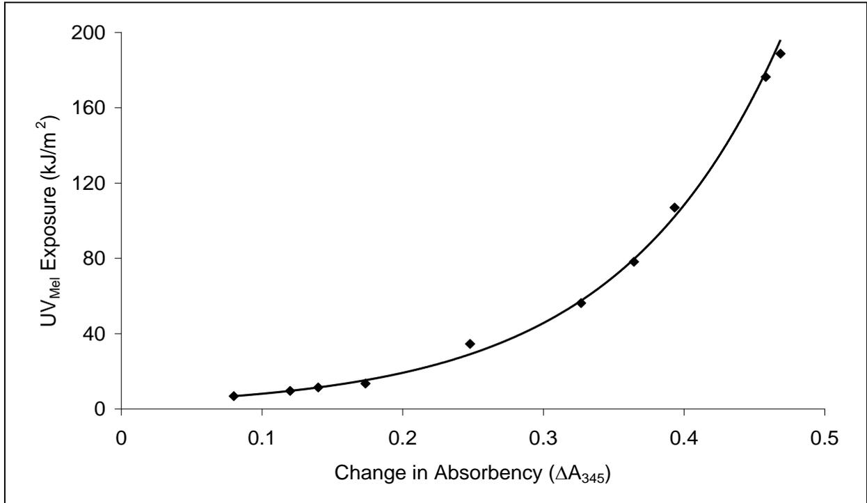
Figure 4. Dose response curve of the UV<sub>Mel</sub> dosimeter for the measurement of the UV<sub>Mel</sub> exposures.
