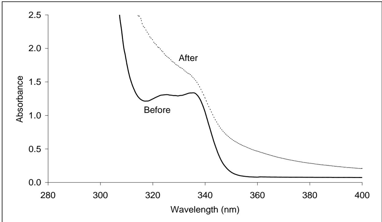
Figure 2. Before and after exposure absorbance characteristics of the UV<sub>Mel</sub> dosimeter after a total UV<sub>Mel</sub> exposure of 190 kJ/m<sup>2</sup>.
