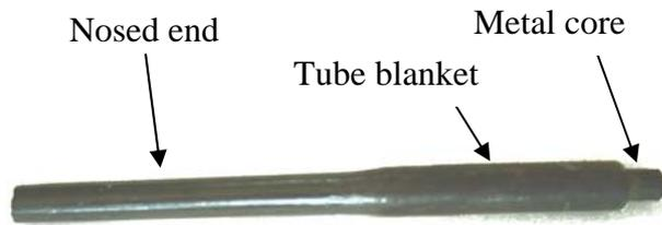
**Fig. 3:** Tube and metal core assembly
