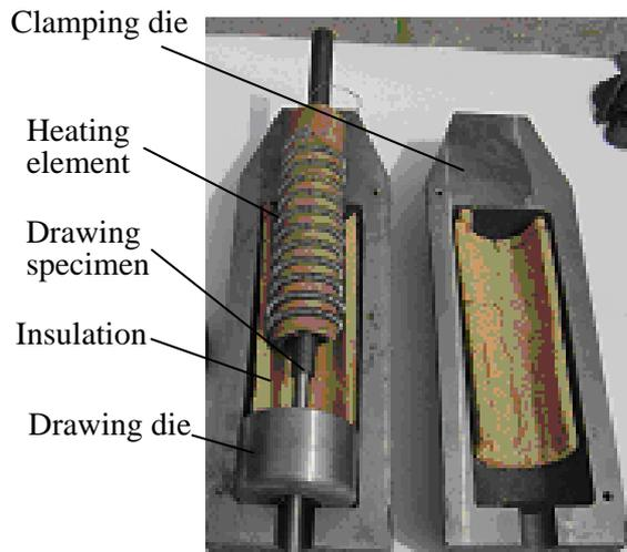
*Fig. 1: Drawing die and clamping die set up*
