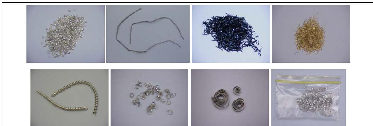
**Figure 4** Chip samples used to enhance tactile appreciation of chip formation and chip packing.
