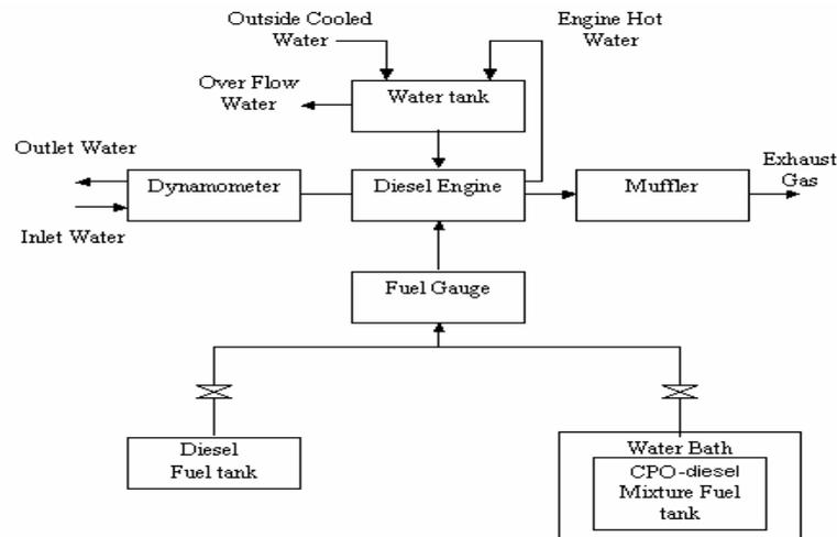
Fig. 1 Schematic layout of the test facilities
