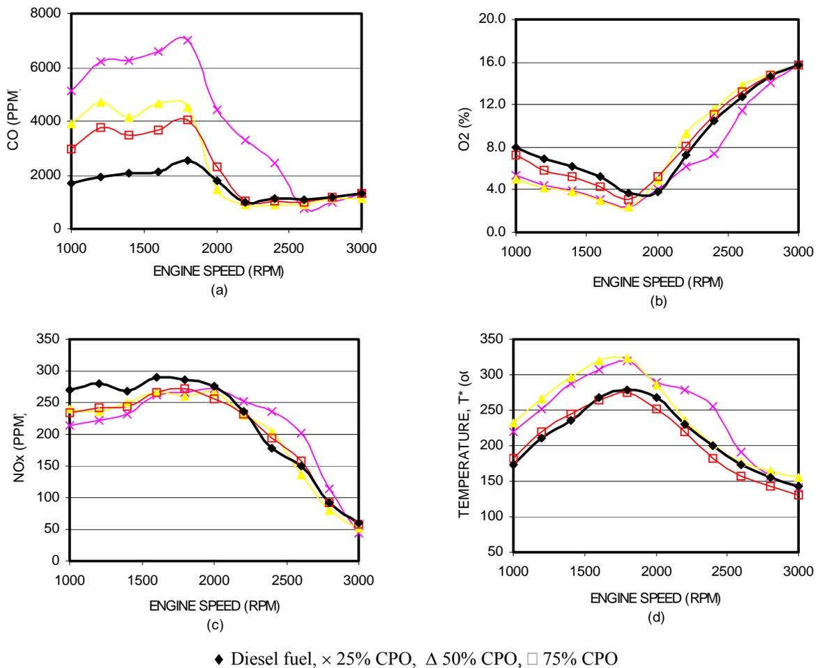
**Fig. 3** Exhaust gas analysis
