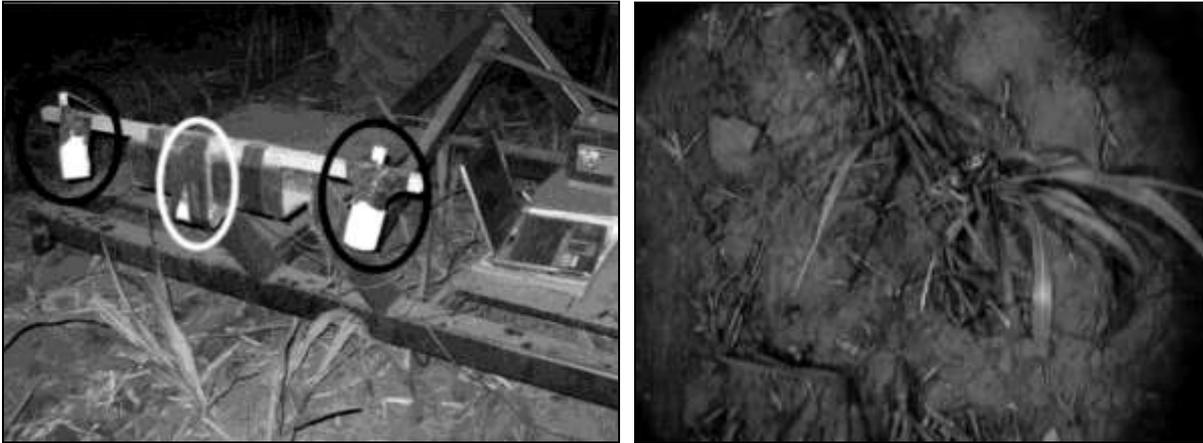
Figure 1. Lighting apparatus for night time trials: (a) equipment setup indicating positions of camera (middle ellipse) and lights (outer two ellipses); and (b) sample image captured at night time (rendered in greyscale).
