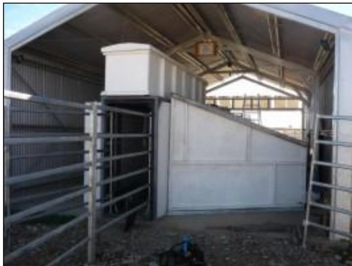
**Figure 6. Apparatus for vision-based cattle condition scoring.**
