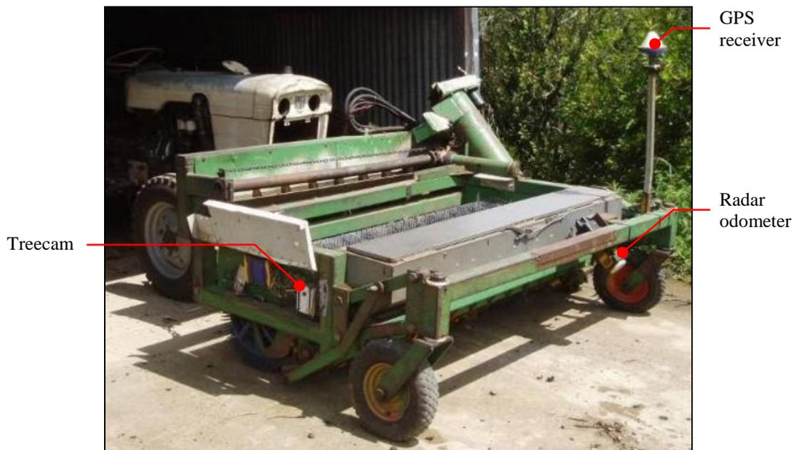
Figure 1. Pinwheel harvester with yield mapping sensors.
