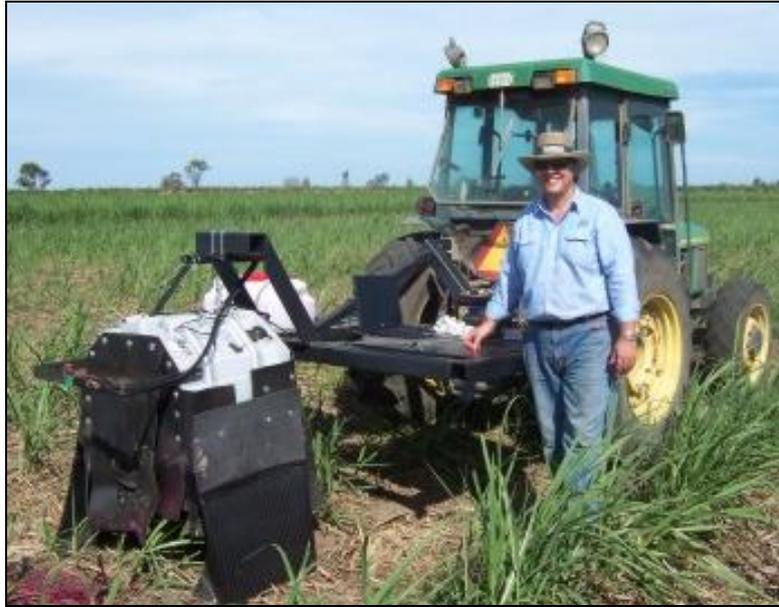
Figure 3. Infield weed spot spraying prototype.
