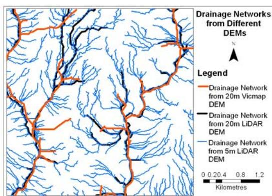
**Figure 5.** Drainage networks from Vicmap DEM and LiDAR DEMs
