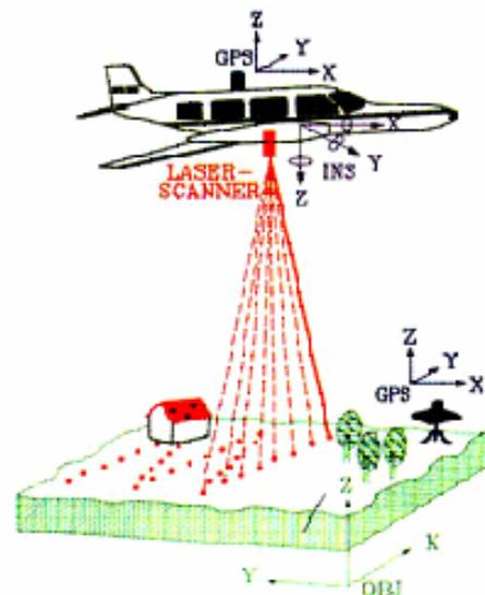
**Figure 1.** A Typical LiDAR System (Gross, 2003)
