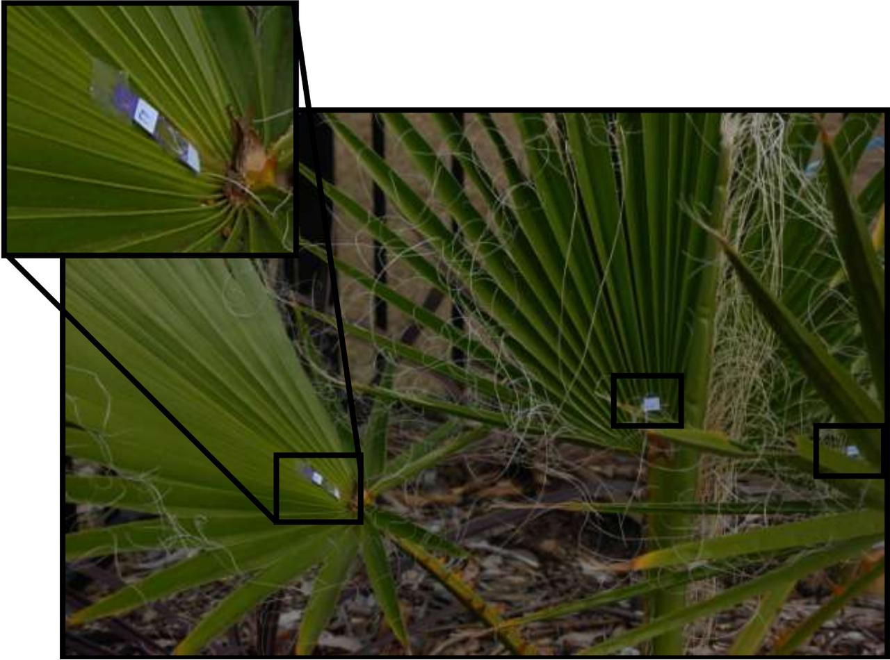
Figure 2 - The miniaturised dosimeters attached to each leaf of a small plant (~0.4 m high) in the field. The dosimeters that are visible are marked with boxes.
