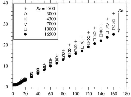
Figure 5: Centerline variation of the mean velocity decay.
