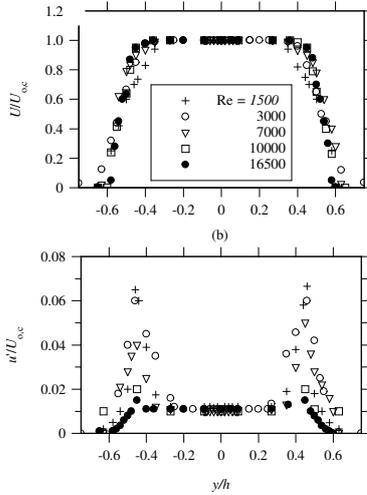
Figure 2: Lateral profiles of (a) normalized mean velocity and (b) turbulence intensity obtained at  $x/H \approx 0.5$ .
