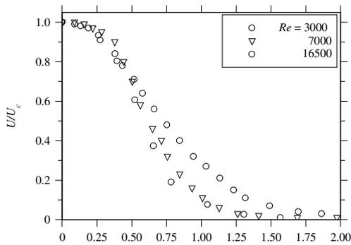
Figure 4: Lateral profiles of  $U/U_c$  at  $x/H = 5$ .
