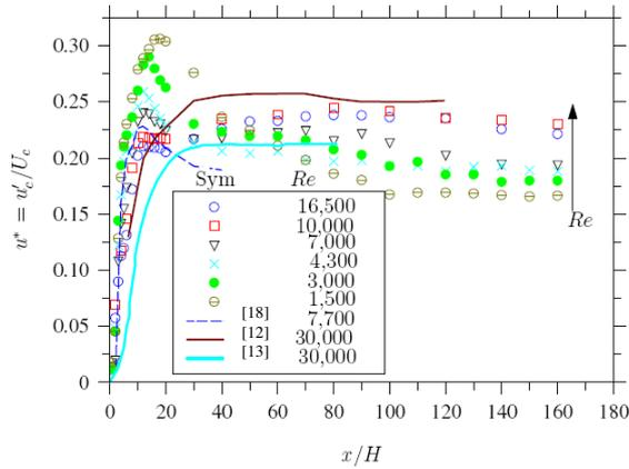
Figure 9: Evolutions of the centerline turbulence intensity.
