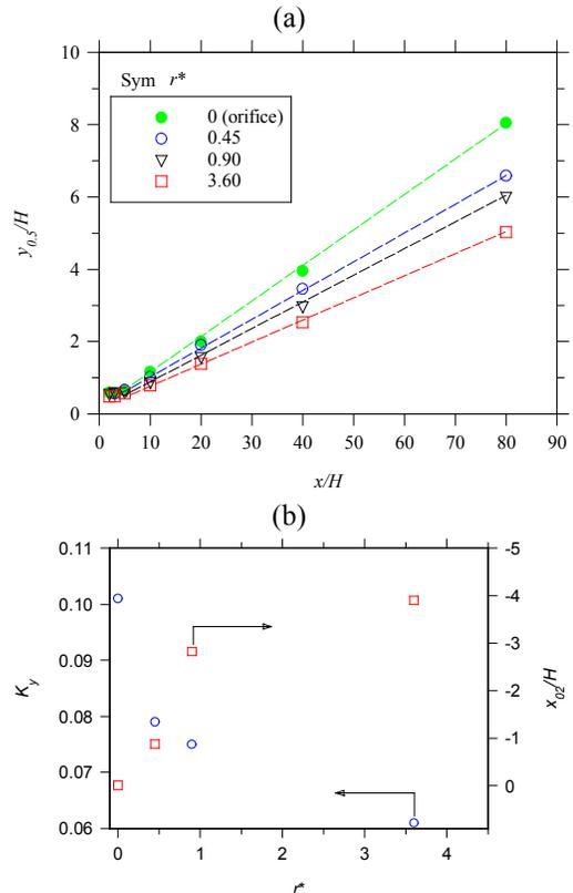
Figure 6 (a) The streamwise variation of the velocity half-width,  $y_{0.5}$  (b) Dependence of the jet spreading rates,  $K_y$  and virtual origin,  $x_{02}/H$  on the  $r^*$
