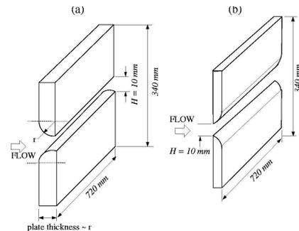
Figure 1. Nozzle plates used for exit profile variation for the cases in (a)  $4.5 \leq r^* \leq 36$  mm, with radial contraction facing upstream and (b) radial contraction facing downstream, i.e.  $r^* = 0$ .
