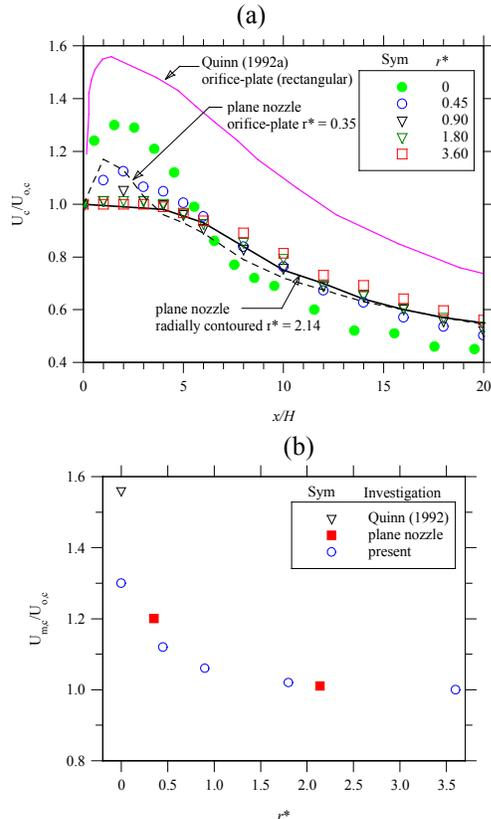
Figure 4 (a) The near field evolution of the normalized mean centerline (b) The dependence of the ratio of the centerline mean velocity maximum,  $U_{m,c}$  to the exit centerline mean velocity  $U_{o,c}$  on  $r^*$  at  $x/H = 3$ .
