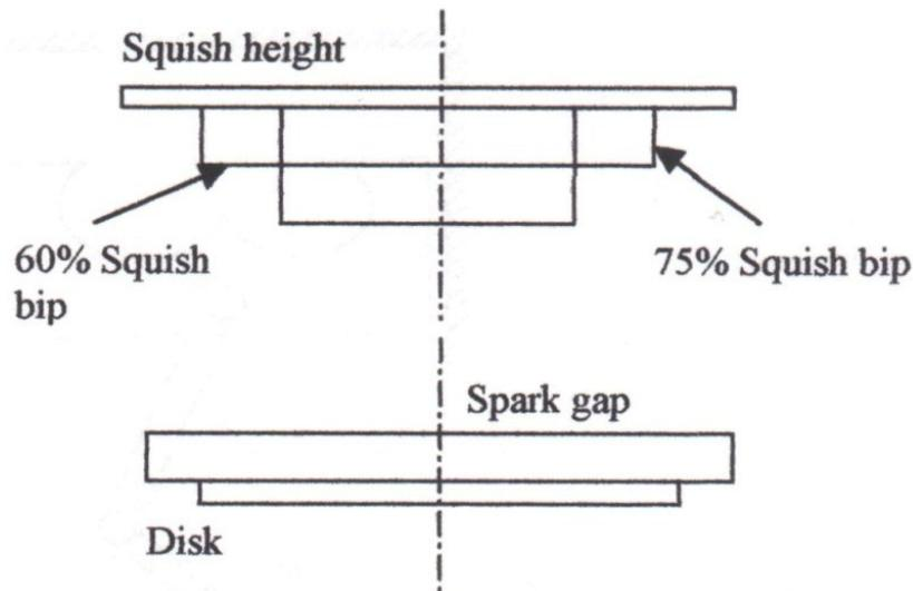
Figure 3.4 – Piston Cup for Swirl Amplification (Ferguson 1986, p. 297)
