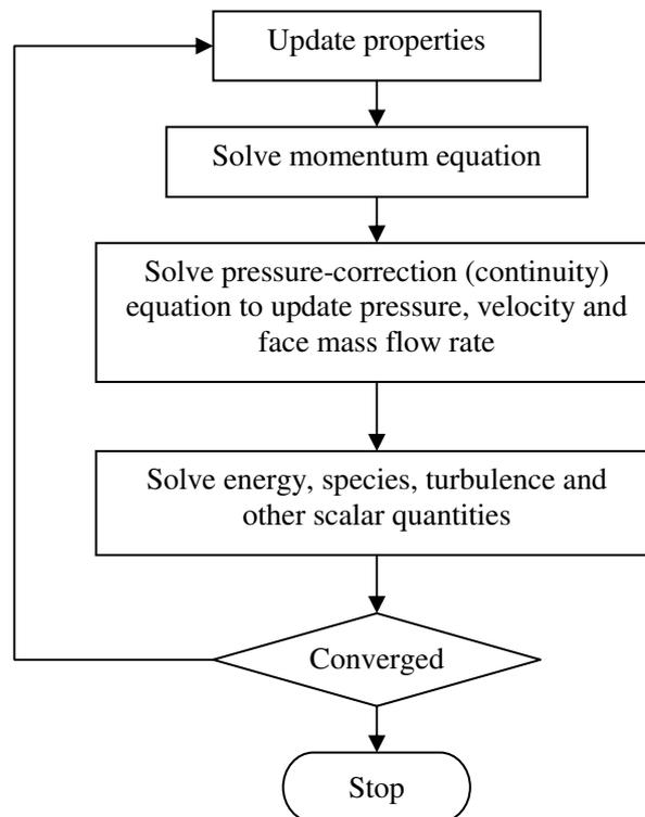
Figure 4.1 – Segregated Solution Loop
