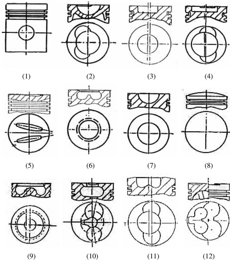
Figure 3.2 - Various Shapes of Piston Crown (KVR BMC Pistons Limited 2004
