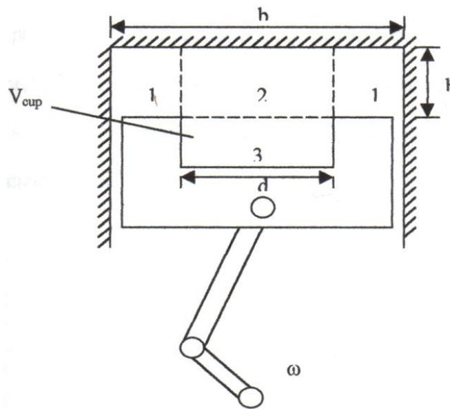
Figure 3.6 – Generation of Squish and Swirl in a Control Volume of a Piston Bowl
