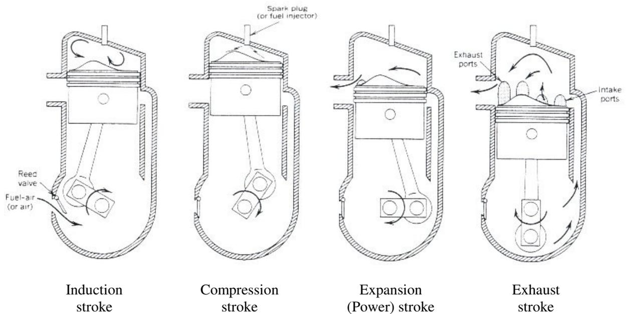
Figure 3.3 - Four-Stroke Cycle (Ferguson 1986, p. 42)
