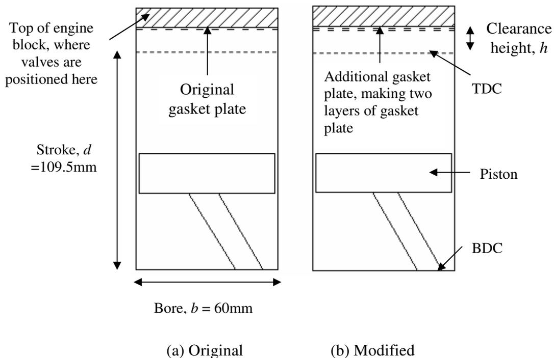
Figure 5.2 – Additional Plate to Increase Clearance Volume
