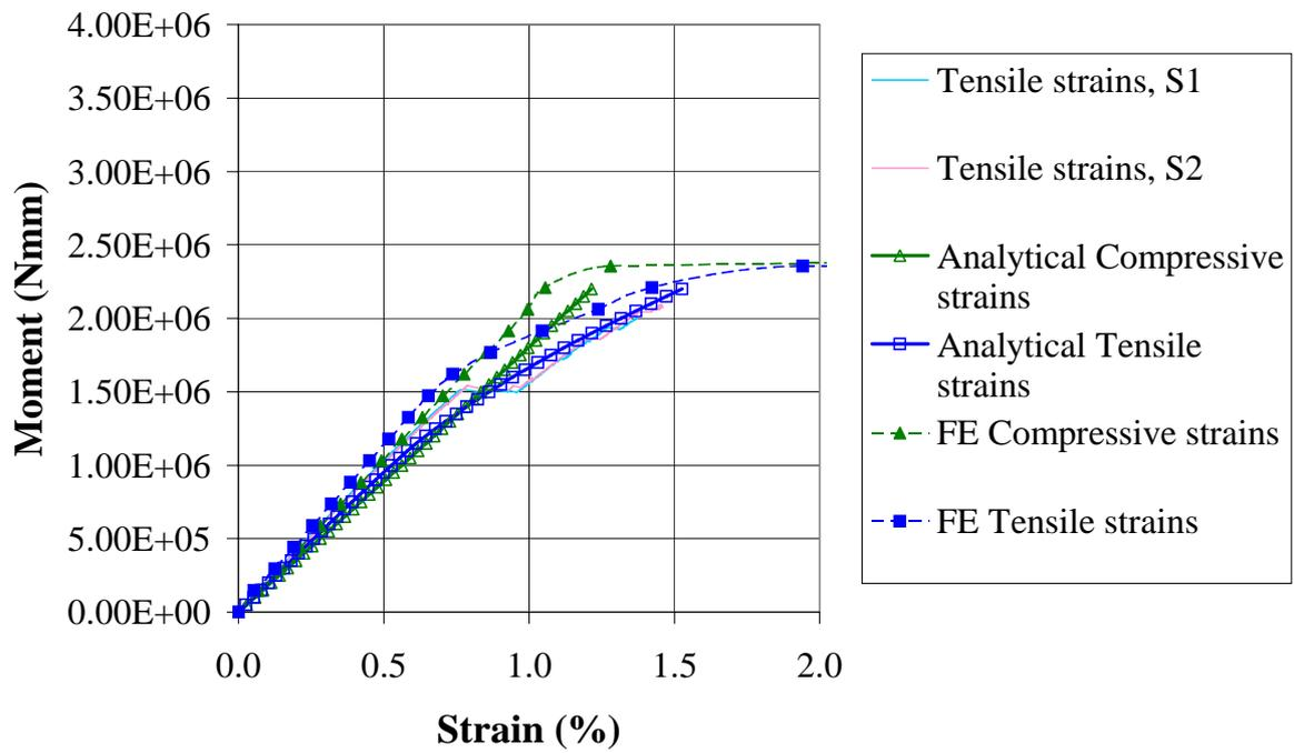
Figure 11: FE versus analytical and experimental results for changing flange core thickness, series B9
