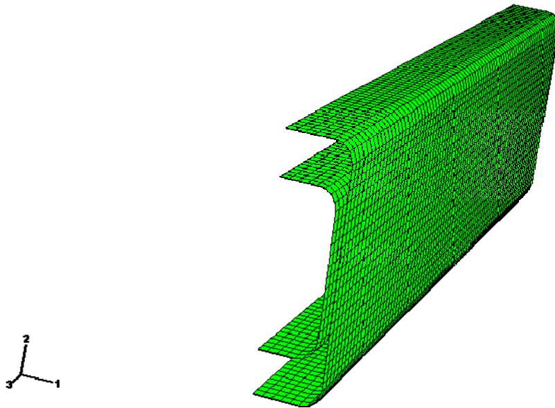
Figure 6: Finite element discretisation of the RHS laminates
