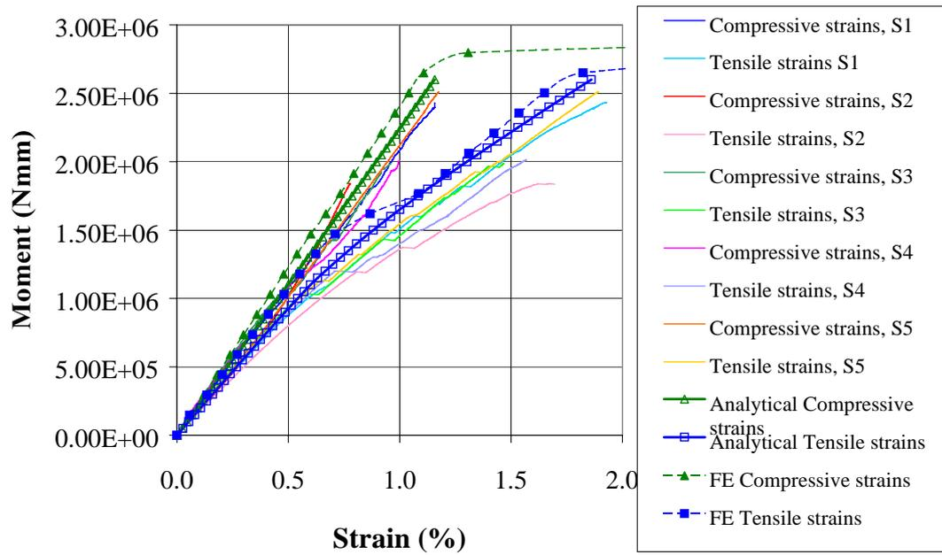
Figure 9: FE versus analytical and experimental results for changing flange core thickness, series B6
