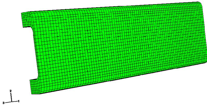
Figure 5: Finite element discretisation of the core and longitudinal laminates
