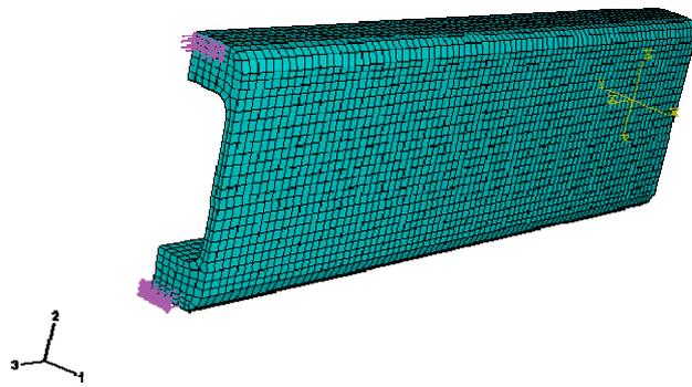
Figure 4: Finite element mesh and loading for pure bending
