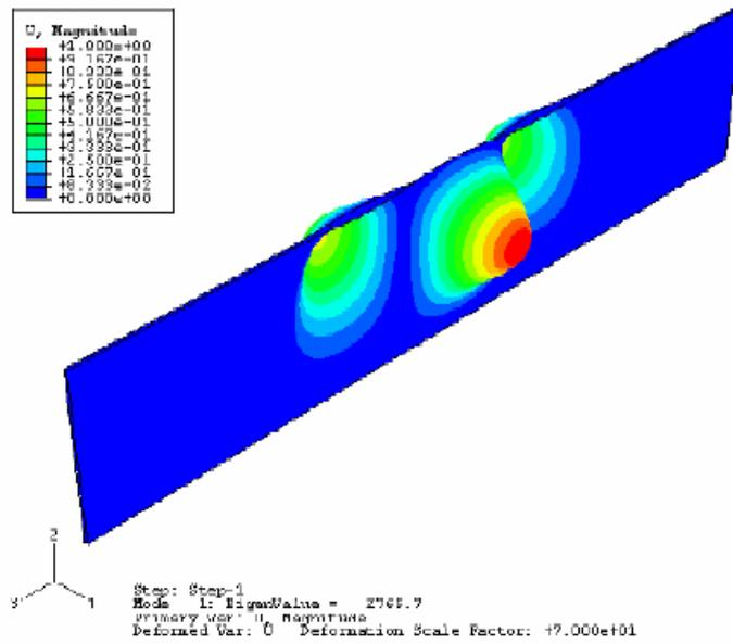
Figure 12: Moment buckling of the web specimen
