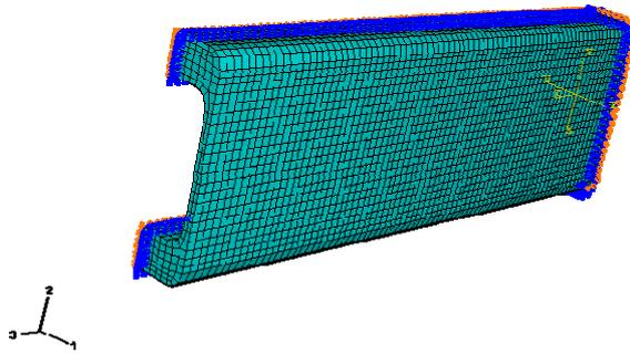
Figure 3: Finite element mesh and boundary conditions for pure bending
