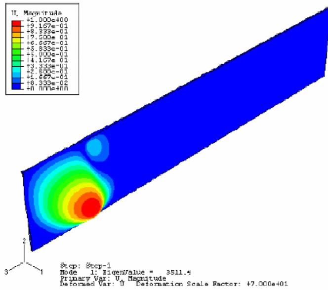
Figure 15: Shear buckling of the web
