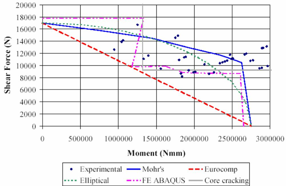
Figure 14: Results for combined shear and bending
