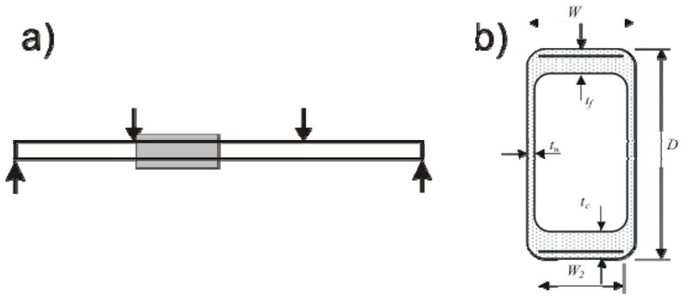
Figure 2: Loading details and cross section .
