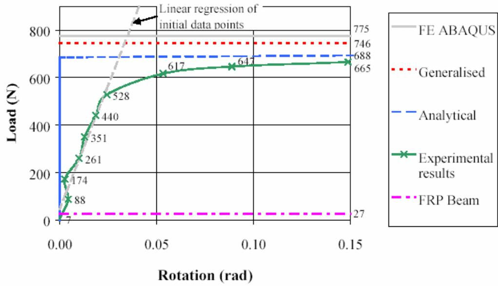
Figure 17: Comparison of lateral torsion buckling predictions
