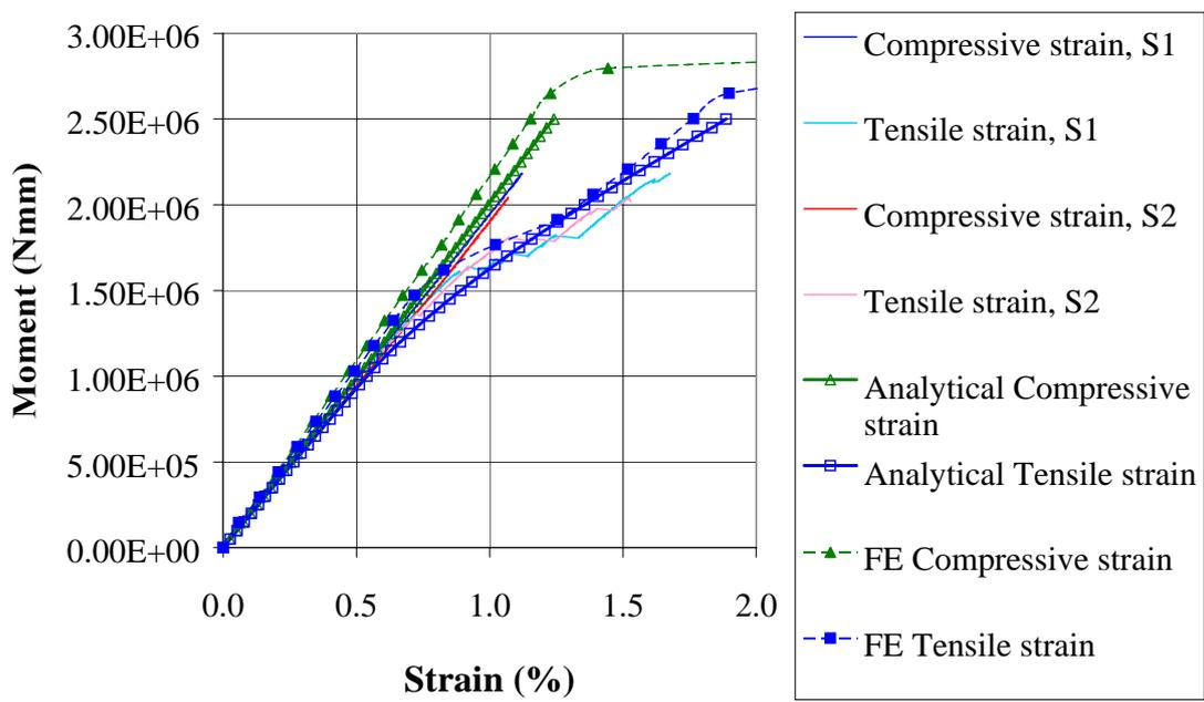
Figure 10: FE versus analytical and experimental results for changing flange core thickness, series B8
