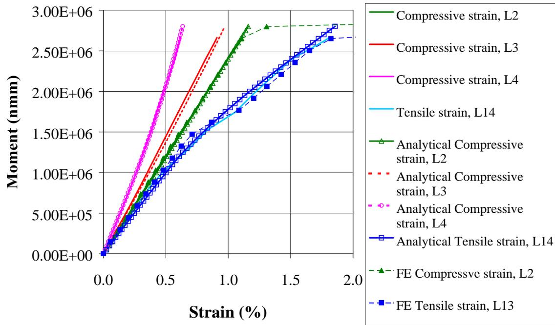
Figure 8: FE versus analytical and experimental results for changing flange core thickness,
