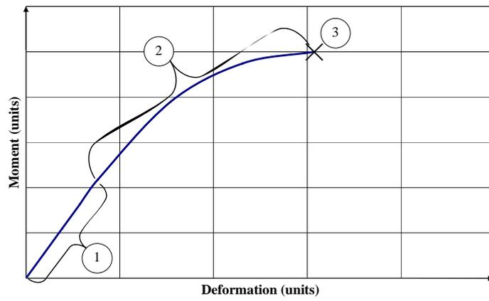
Figure 2: load deformation behaviour of a composite beam incorporating core material
