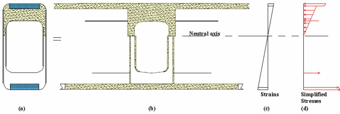
Figure 6: Transformed section of cracked FRP beam
