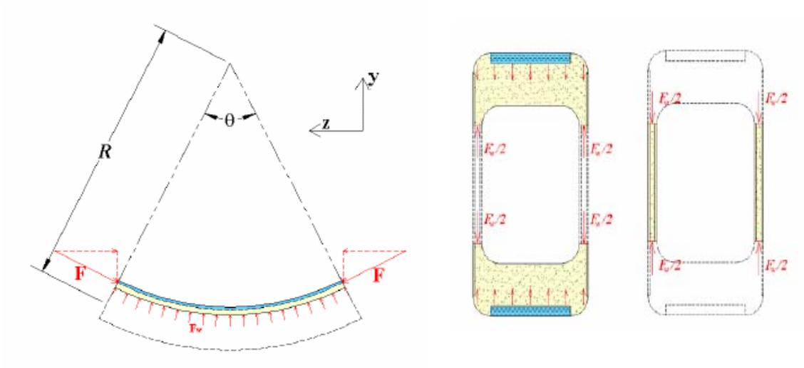
Figure 9: Secondary forces in webs induced by bending or applied external force
