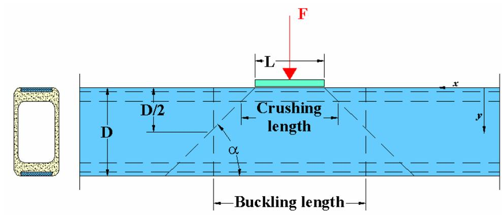
Figure 8: Vertical compression forces in the webs generated by an externally applied load
