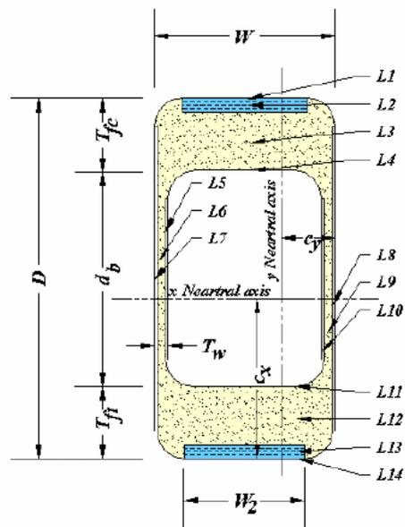
Figure 1: Three dimensional view and cross section of the beam prototype
