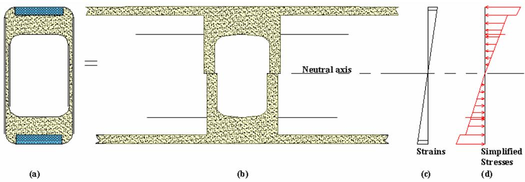
Figure 3: Transformed section of the un-cracked FRP beam
