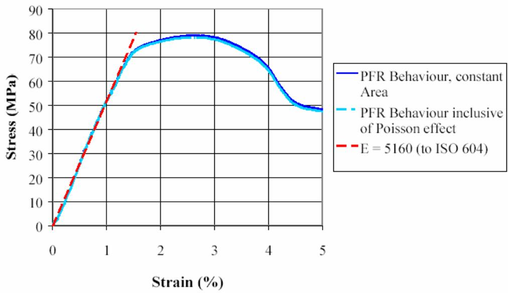
Figure 5: Stress-strain behaviour of the PFR material in compression
