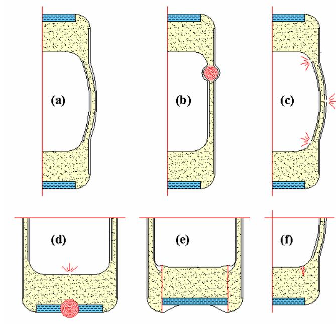
Figure 7: Some secondary failure modes in bearing
