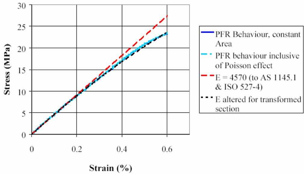
Figure 4: Stress-strain behaviour of the PFR material in tension
