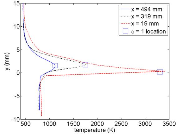
Figure 5. Profiles of temperature at 3 locations downstream of the splitter plate.
