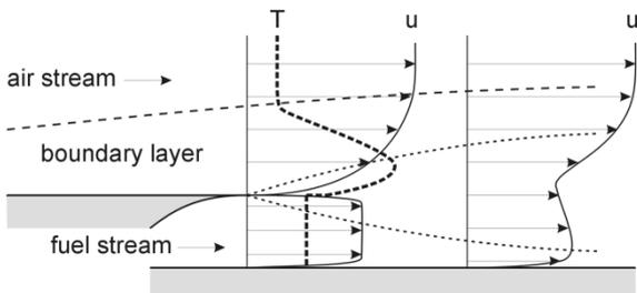
Figure 2. Illustration of mixing layer development in the presence of a boundary layer.
