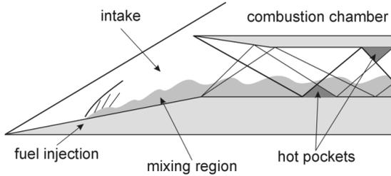
Figure 1. Schematic illustration of a scramjet intake and combustion chamber.
