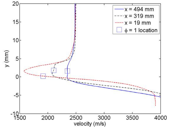
Figure 6. Profiles of velocity at 3 locations downstream of the splitter plate.
