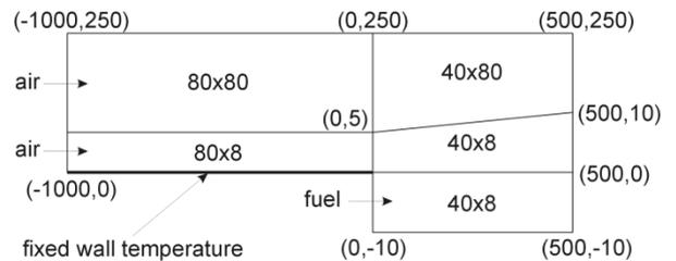
Figure 3. Blocks used in numerical simulation, not to scale. Number of cells in each block is given by  $n_x \times n_y$  near the centre of each block and the position of selected corners are given by  $(x, y)$  with numerical values reported in mm.
