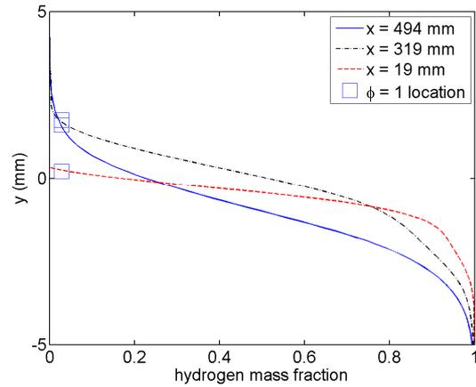
Figure 4. Profiles of hydrogen mass fraction at 3 locations downstream of the splitter plate.
