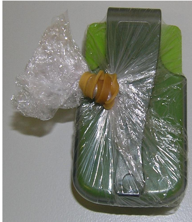
Figure 2: The Edison handheld solar UV meter covered in glad wrap front view (A) and back view (B).
