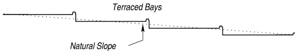
Longitudinal Cross-Section (b)
