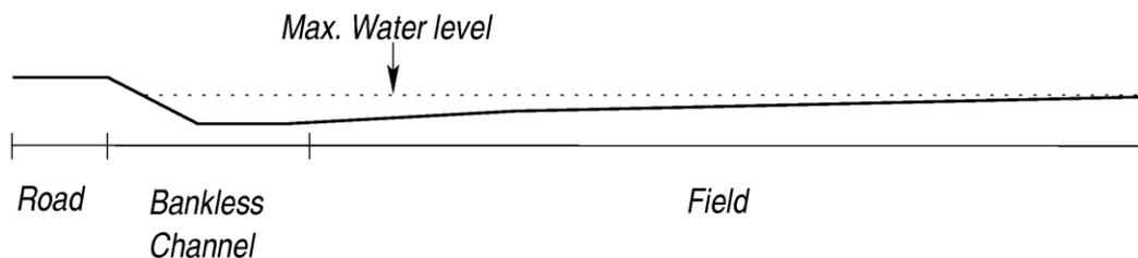
**Figure 1:** Schematic of bankless channel irrigation system.
