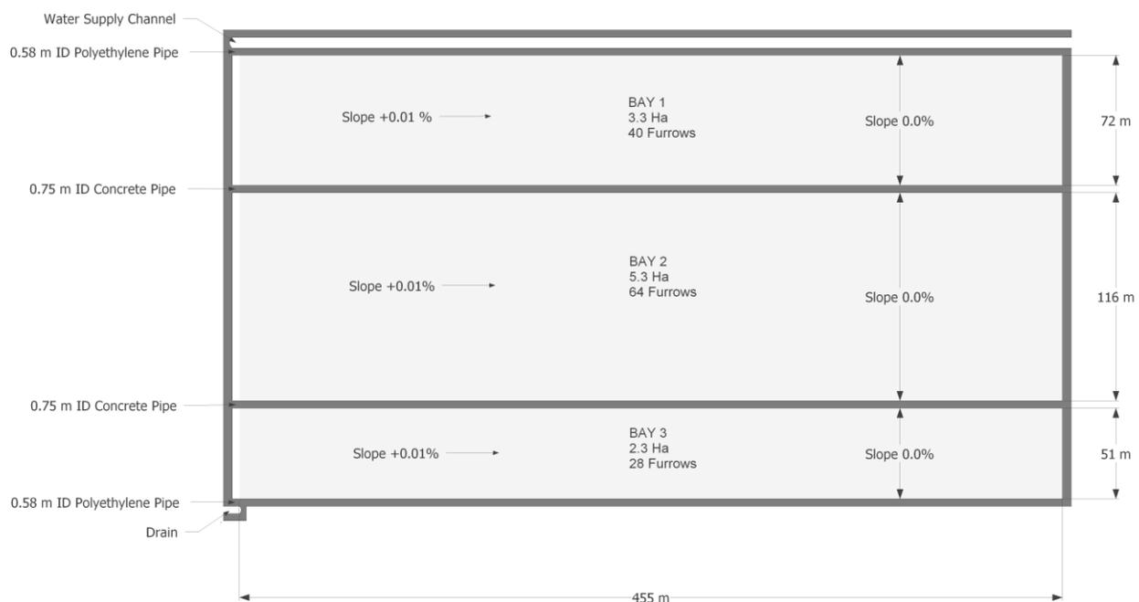
**Figure 2:** Dimensions, bay area and key features of the field selected for evaluation. Irrigation water is supplied to the field via the supply channel above Bay 1. Pipes connect the supply channel to the bankless channel which distributes the water across the inlet width of the field. A 0.15m step exists between bays, such that bay 3 is lower than bay 2 which is in turn lower than bay 1.
