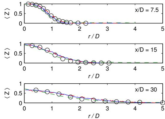
Figure 1: Favre-averaged mixture fraction profiles at various stations. Hybrid binomial Langevin–MMC, —; EMST ( $C_\phi = 2.0$ ) (current), —; EMST ( $C_\phi = 2.0$ ) [16], - -; Experiment [9],  $\circ$ .
