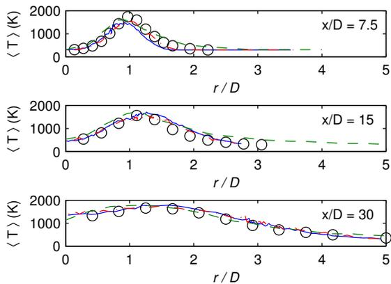
Figure 2: Favre-averaged temperature profiles at various stations. As per Fig. 1.
