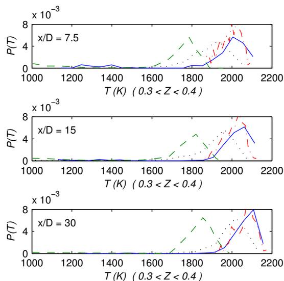
Figure 4: Conditional PDFs of temperature, conditioned on mixture fraction. Hybrid binomial Langevin–MMC, —; EMST ( $C_\theta = 2.0$ ) (current), - -; EMST ( $C_\theta = 1.5$ ) [16], - · -; Experiment [9], ···.
