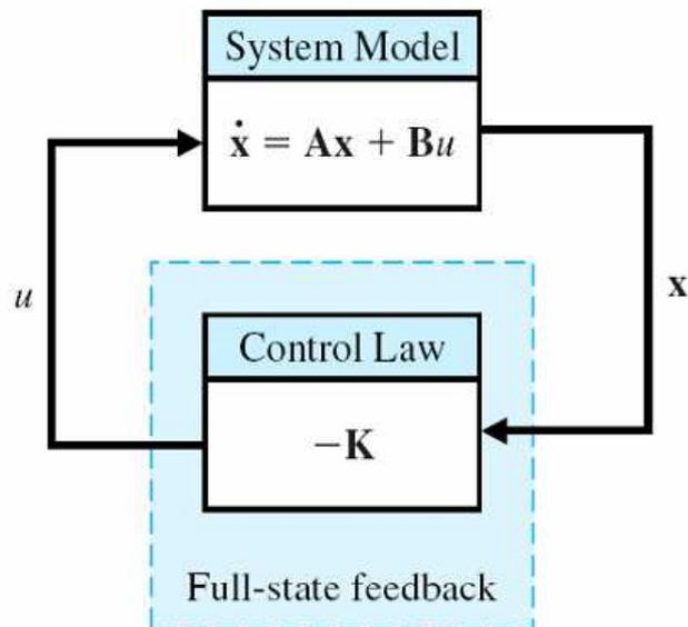
Figure 2.2: Linear-State Feedback System [3]
