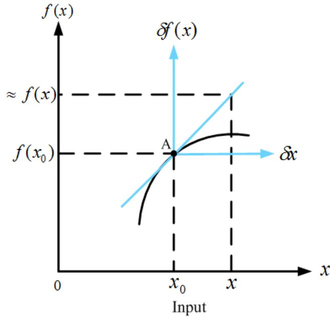
Figure 2.1: Non-linear System Linearised about Point A
