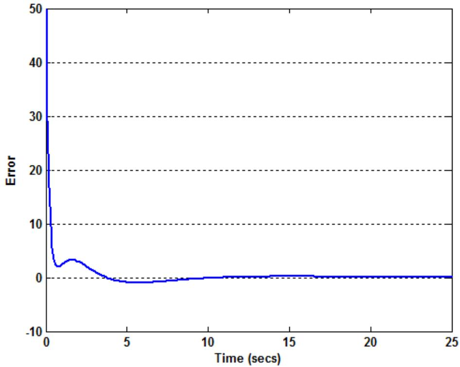
Figure 5.14: Observer Error of Functional Observer
