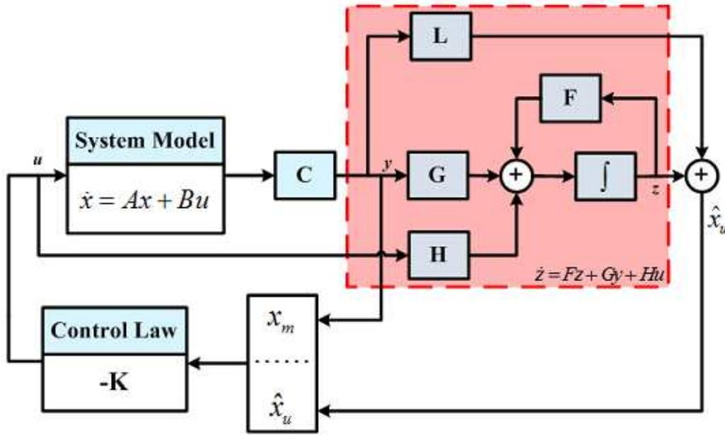
Figure 3.3: Schematic of a Reduced-Order Observer
