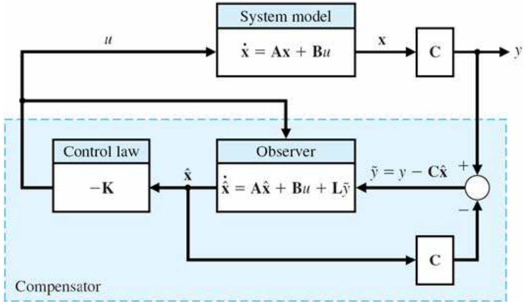
Figure 3.2: Schematic of a Full-Order Observer [3]
