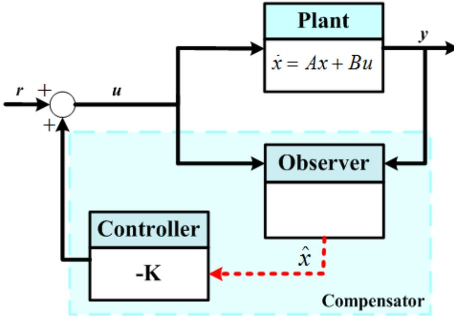
Figure 3.1: Closed-loop Observer for State Feedback
