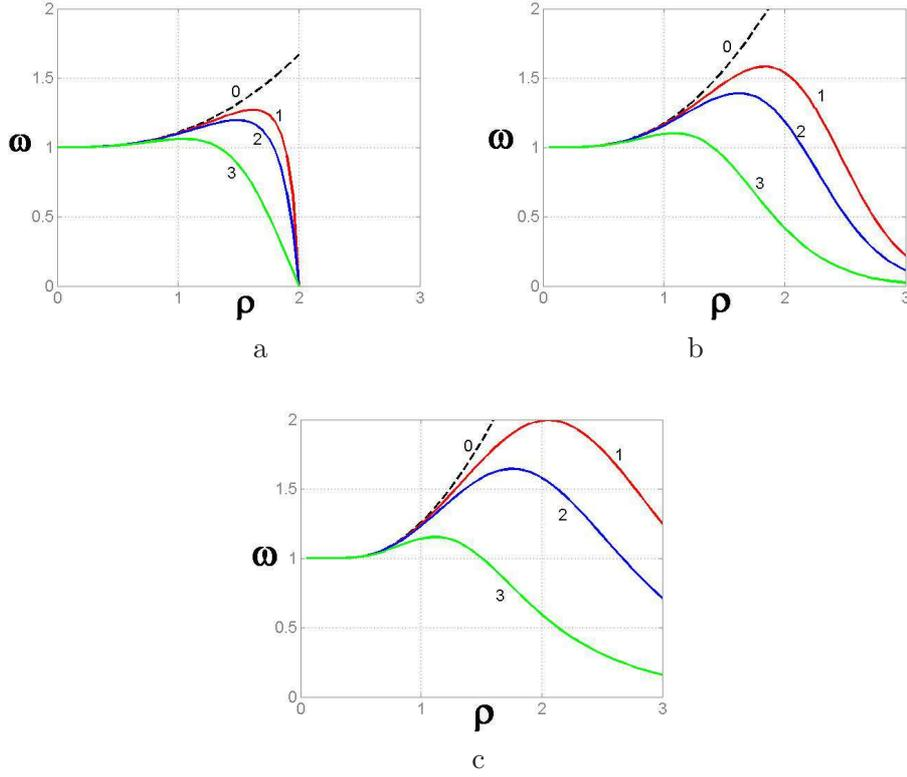
Figure 3. Velocity enhancement factor,  $\omega(\rho, C)$ , versus normalized particles radius  $\rho$  at various colloid concentrations  $C$  for the uniform (a), Rayleigh (b) and log-normal (c) distribution of tube radii. Dashed lines (0) correspond to the ideal enhancement factor. Solid lines: (1)  $C = 0.05$ ; (2)  $C = 0.1$ ; (3)  $C = 0.5$ .
