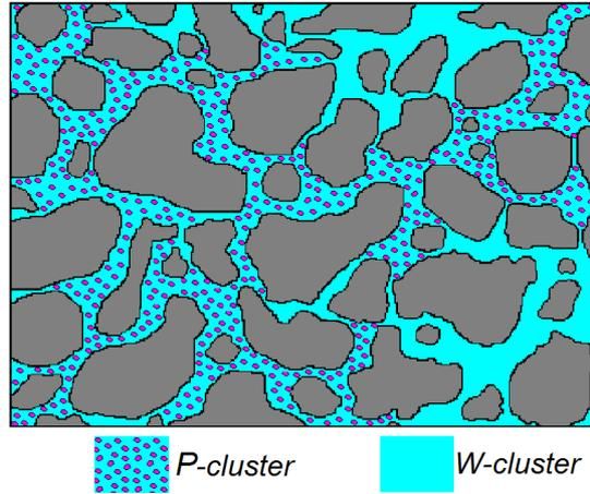
Figure 6. Two clusters of pores: P-cluster is occupied by particles, while W-cluster contains only pure water.
