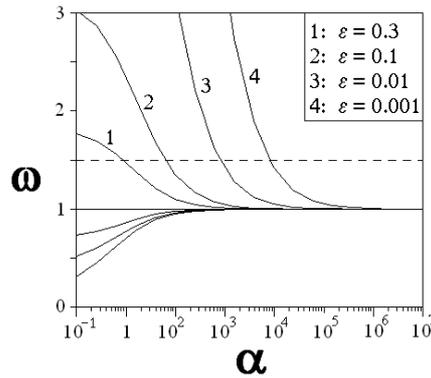
Figure 11. Radionuclide velocity enhancement factor versus relative concentration of particles  $\alpha = N_1/N_2$  for several values of particle mass ratio  $\varepsilon$
