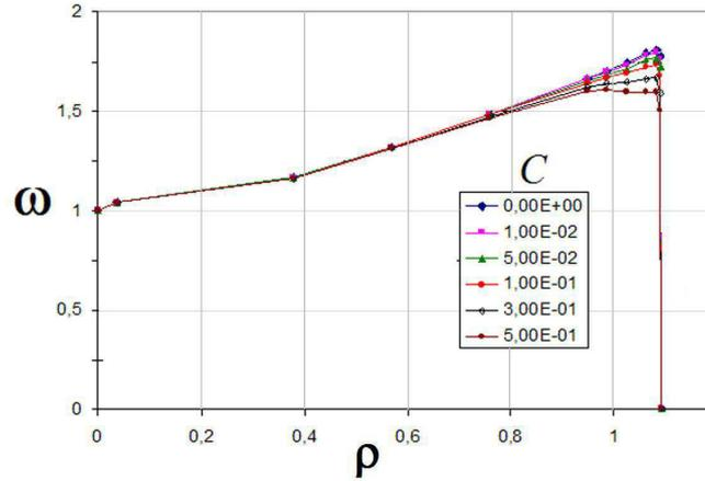
Figure 8. Enhanced factor  $\omega$  vs. dimensionless particle radius  $\rho$  for various concentrations  $C$ .
