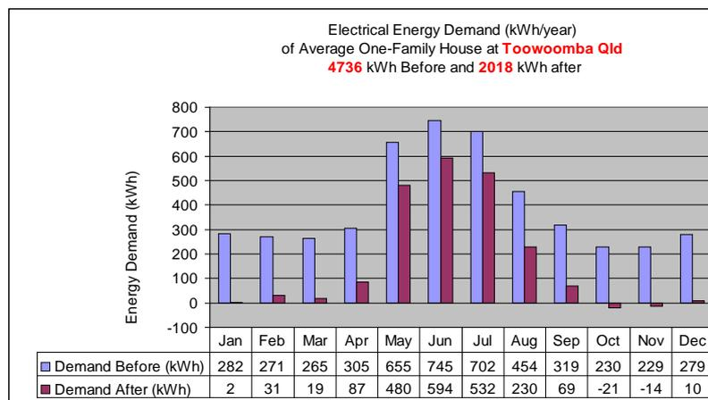
Figure 4. Electric energy savings from the PV-SWH combined solar system.
