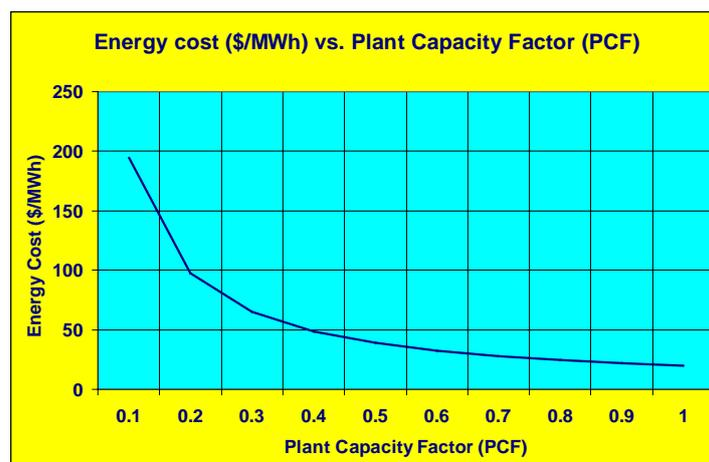
**Figure 6** Impact of the plant capacity factor on the cost of the produced energy.
