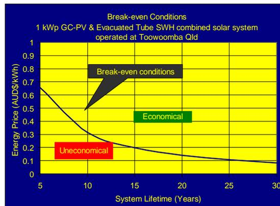
**Figure 5.** Break-even conditions of the 1 kW GC-PV operating alongside a 1.37m<sup>2</sup>/120 Litre evacuated tube SWH system.
