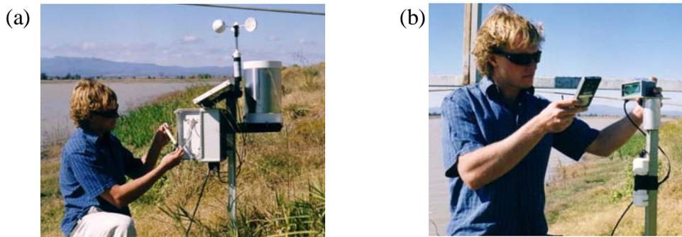
**Figure 3.** The Irrimate™ (a) storage calibration meter and (b) storage volume meter
