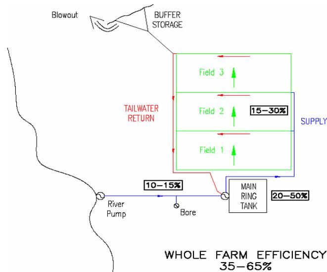
**Figure 1.** Typical water balance for whole farm irrigation flows (common volumetric losses shown in boxes)
