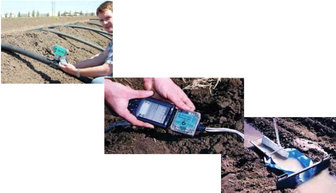
**Figure 6.** Irrimate™ surface evaluation equipment (a) inflow meter, (b) advance sensors and (c) flumes
