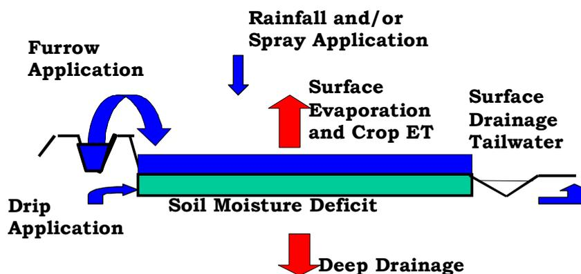
**Figure 5.** Components of the in-field application system volume balance
