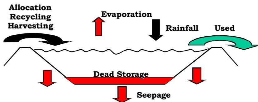
**Figure 2.** Components of the water storage volume balance
