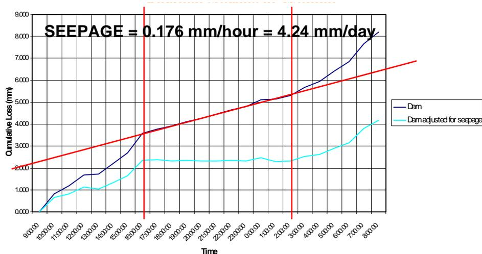
**Figure 4.** Seepage measurement using logged pressure depth sensors
