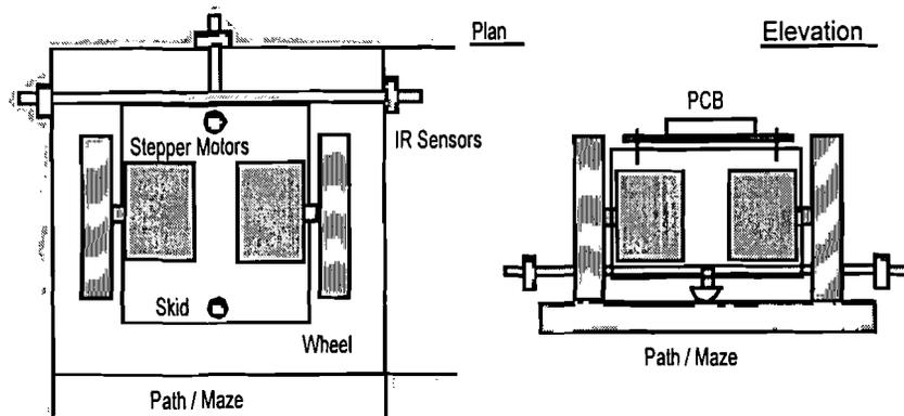
Fig 2. Plan and elevation of the kit Bilby Robot.
