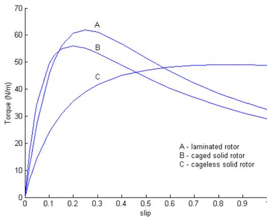
Figure 3: Torque-Speed Characteristics
