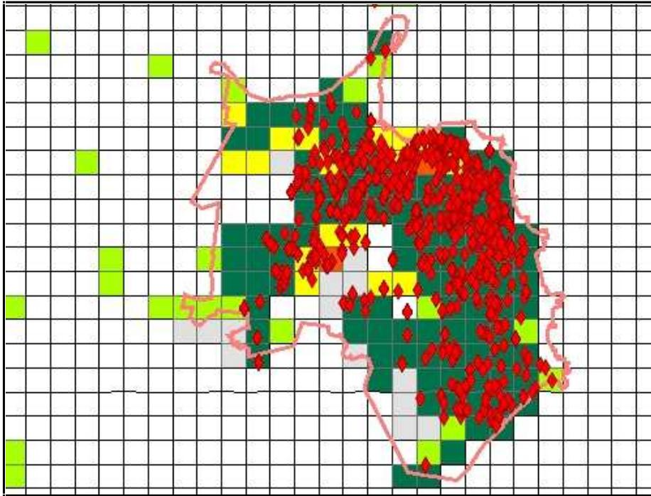
Figure C.5 Combined hazard and likelihood layers for Port Macquarie showing no correlation between incidents and hazards
