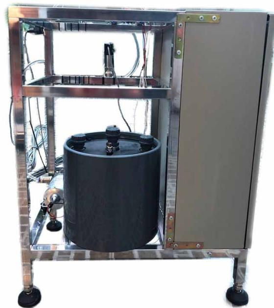
**Figure 2** | MCDI pilot plant for desalination including the electrode module (Voltea C3) and power supply (XP Power HDS 1500 PS12).
