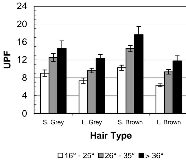
Figure 5 – The UPF for the upright head in full sun for each hair type averaged for the SZA ranges of 16 – 25 degrees, 26 – 35 degrees and greater than 36 degrees. The error bars represent  $\pm$  one standard error.
