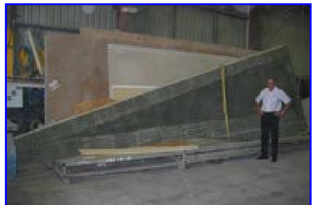
Figure 3. Fibre composite windmill tower after joining faces using corner angles
