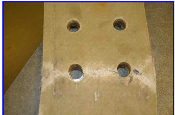
Figure 11. Failure modes for the tested brackets
