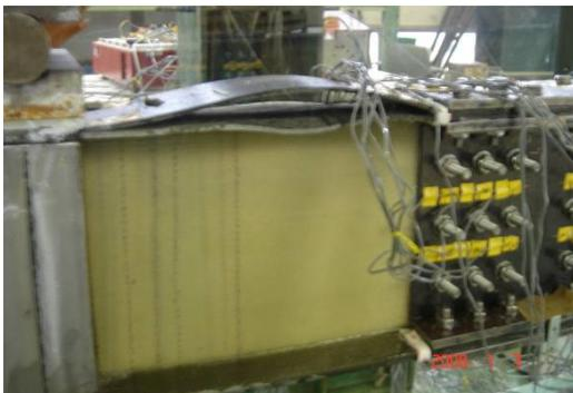
Figure 13. Failure mode of hybrid FRP girder with bolted and epoxy bonded joints
