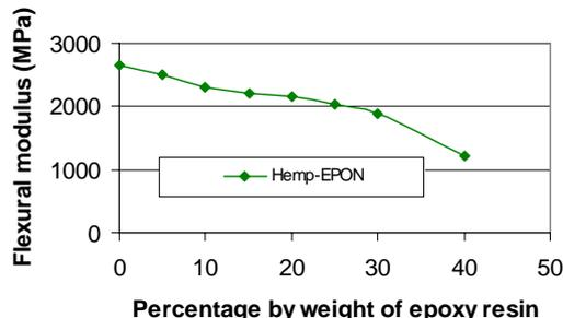
Figure 2. Flexural modulus vs. percentage of Hemp-EPON
