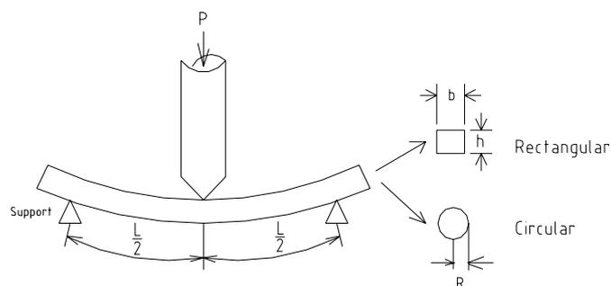
Figure 1. A schematic diagram for three point bending test.
