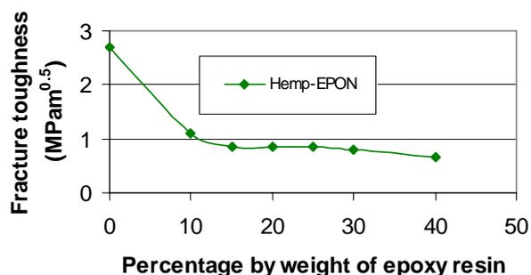
Figure 4. Fracture toughness vs. percentage of Hemp-EPON
