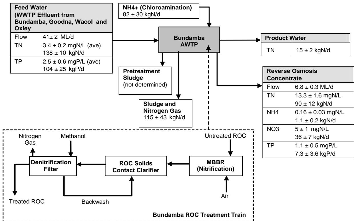
**Figure 3:** Nutrient mass balance for Bundamba AWTP – August 2008 to February 2009.
