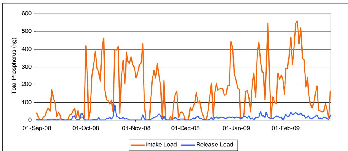
**Figure 4:** Luggage Point AWTP - daily intake and release loads of total phosphorus (kg).
