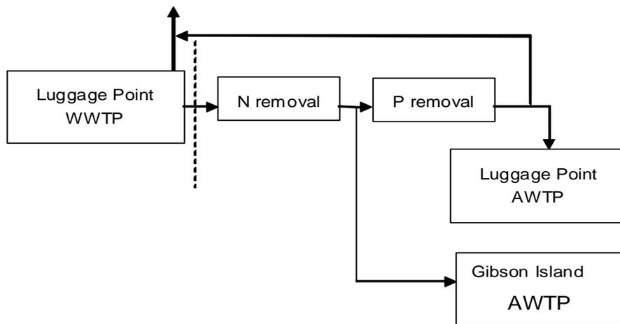
**Figure 5:** Option for pretreatment reduction of Luggage Point treated wastewater nitrogen loads.
