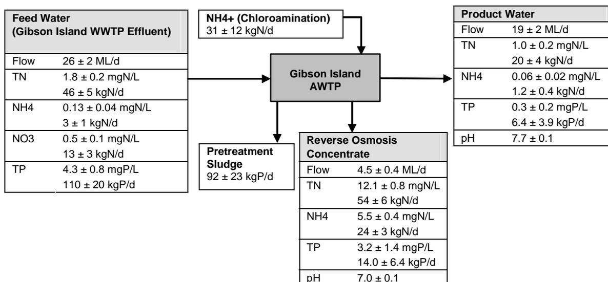
Figure 2: Nutrient mass balance for Gibson Island AWTP – August 2008 to February 2009
