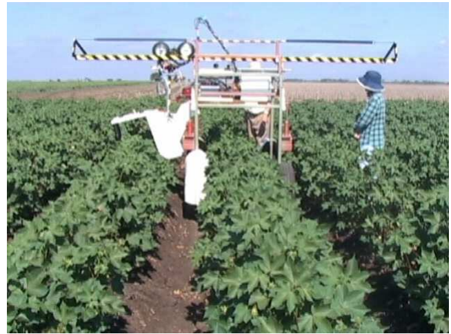
Fig. 4. Vehicle for scanning internode length
