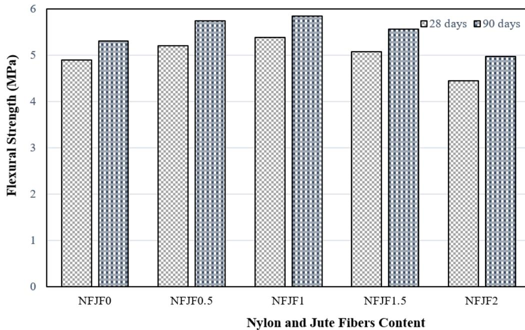
**Figure 9.** Flexural strength of concrete.
