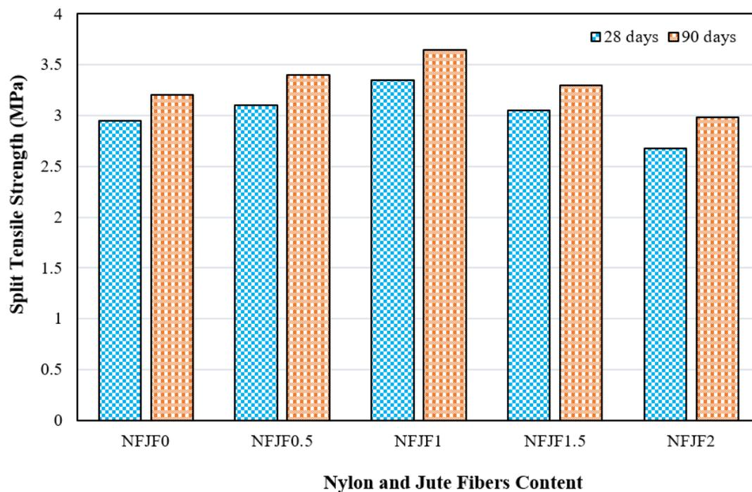
**Figure 8.** Splitting tensile strength of concrete.
