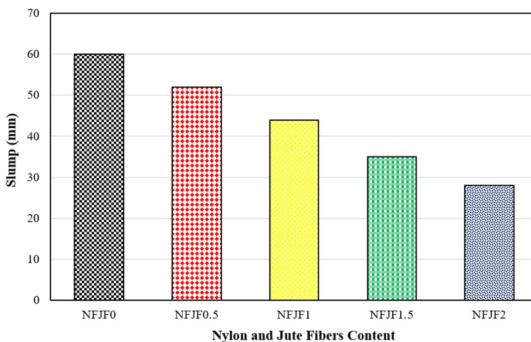
Figure 4. Slump test.
