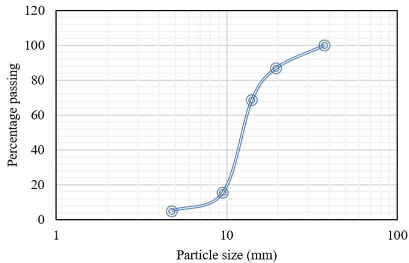
**Figure 1.** Grading curve of coarse aggregate (CA).
