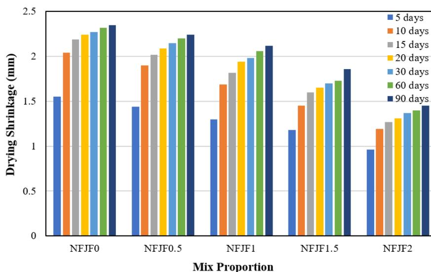
Figure 11. Drying shrinkage of concrete.
